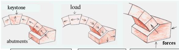
The load at the top of the key stone makes each stone on the arch of the bridge press on the one next to it. This happens until the push is applied to the end supports or abutments, which are enbedded in the ground.
