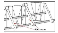
A **buttress** is a structure built against or projecting from a wall which serves to support or reinforce the wall.
