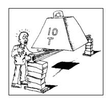
A **cantilever** is a structural member which sticks out like an arm form the main structure. A cantilever is a beam which is supported at one end only.
