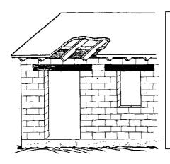
Lintels are beams made of concrete and reinforced with steel bars. They spread the weight of the structure above the opening of doors and windows to the structure beside them.
