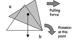
If the structure is stable, on release of the pulling force the structure will return to its original position.
