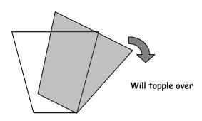
However, it must be noted that this will only be the case if the centre of gravity remains inside the base of the structure. When the structure is tilted to such a degree that its centre of gravity is outside its base, then the structure will become unstable as gravity acts on it and causes it to topple over.
