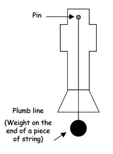
Repeat the process again twice, but each time place the pin at a different location, and mark the position of the plumb line string. Where the three pencil lines cross is the centre of gravity of the shape.
