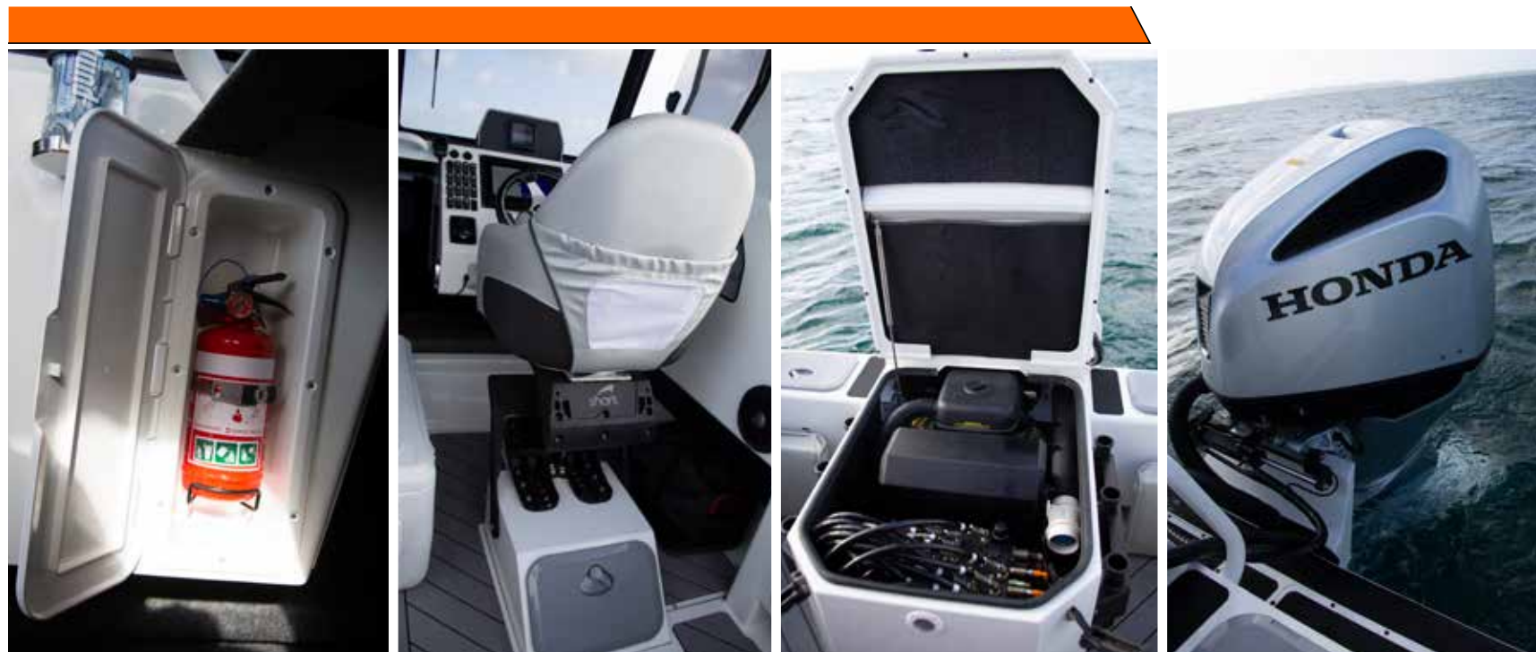
From left: Even the fire extinguisher has its own dedicated locker; Two Shark hydraulic seats make for a comfortable ride for the skipper and the navigator; The Orion's power source – it will run for as long as there is fuel, never overheating; The economy of the latest Honda 250 D outboard coupled with a 200-litre underfloor tank gives the boat a big range.
