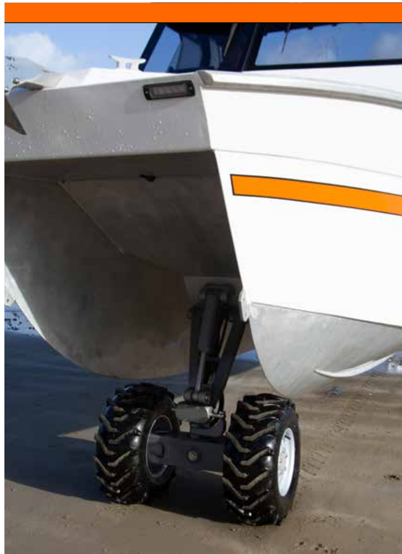
Left: The Orion system spreads the weight of the boat over four driving wheels. The clip-on gunwale is an innovation that allows owners to choose between two gunwale heights depending on their needs.
