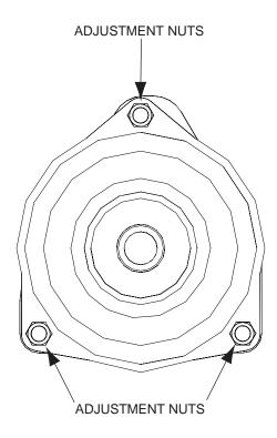
Figure 6-11. Clutch Air Gap Adjustment
