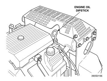
Figure 7-4. engine Oil Fill/Dipstick Location
