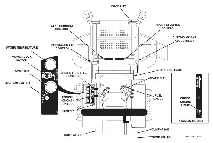
Figure 4-1. Controls and Instruments
