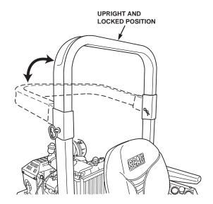
Figure 2-1. Foldable Roll-Over Protection System
