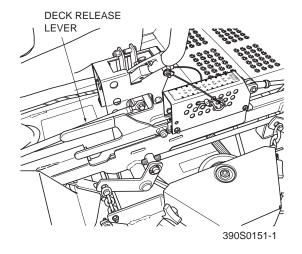
Figure 4-6. Deck Release Lever
