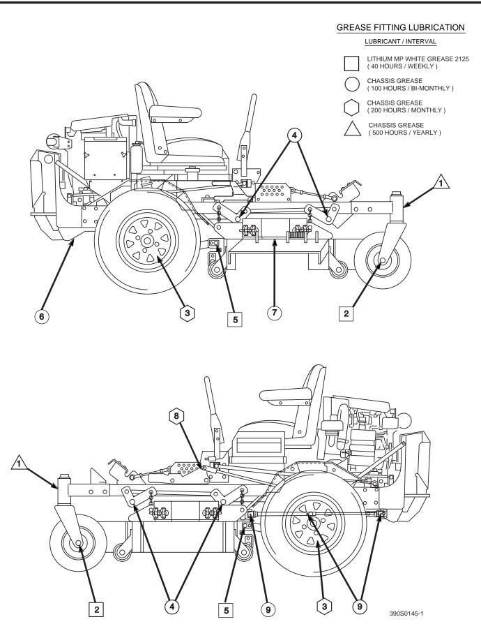
Figure 7-1. Lubrication Fitting Points
