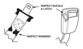
Figure 2-3. Seat Belt Inspection
