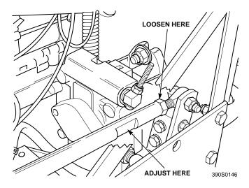
Figure 6-4. LH Steering Control Rod Adjustment
