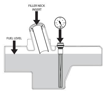
Figure 7-6. C.A.R.B. / e PA Phase 3 Fuel Level
