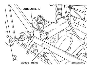
Figure 6-3. RH Steering Control Rod Adjustment
