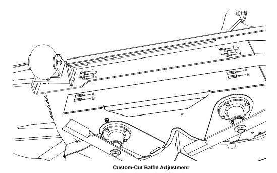
**Mounting Slot Selected Mounting Hardware Location** Slot "A" Hole 3 Hole 4 Hole 1 Hole 2 Height (inches) 3-3/4" 4-1/4" 4-3/4" 5-1/4" Slot "B" Hole 2 Hole 3 Hole 4 Height (inches) 3-1/2" 4-1/2"
