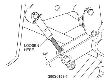
Figure 6-2. Brake Rod Adjustment
