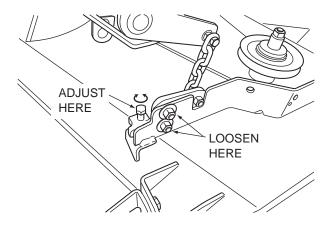
Figure 6-5. Cutter Deck Level Adjustment
