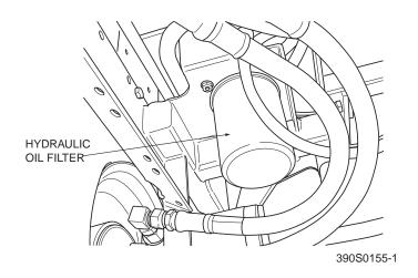
Figure 7-3. Hydraulic Oil Filter
