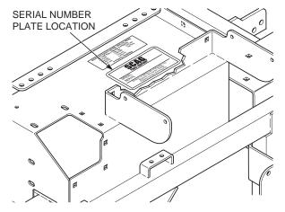
Figure 1-1. Mower Serial Number Plate Location
