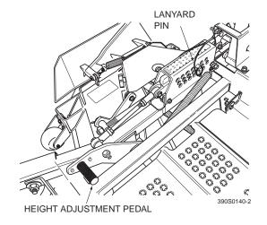
Figure 4-5. Adjusting Cutting Height
