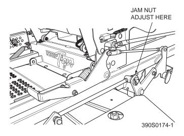
Figure 6-6. Cutter Deck Level Adjustment
