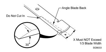
Figure 7-8. Blade Sharpening
