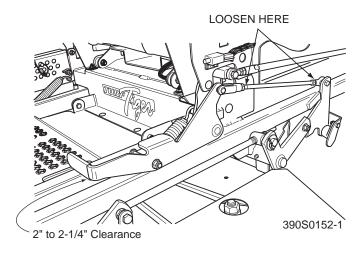
Figure 6-1. Brake Adjustment
