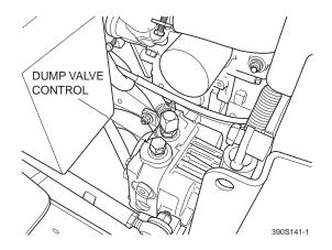
Figure 4-4. Dump Valve Control
