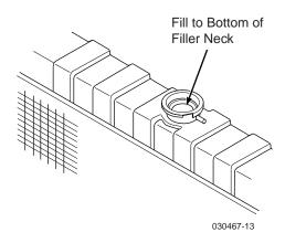
Figure 7-11. Coolant Level
