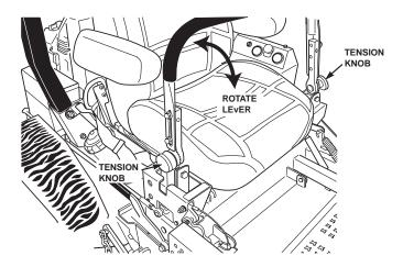
Figure 4-7. Adjusting Steering Levers
