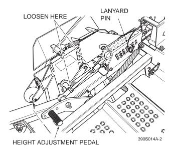
Figure 6-7. Cutter Deck Height Adjustment
