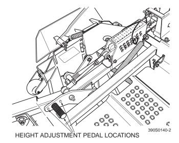
Figure 4-8. Height Adjust Pedal Locations
