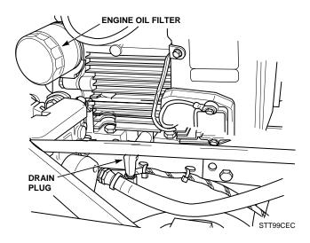
Figure 7-5. Drain Plug and Oil Filter Location
