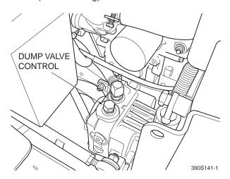
Figure 4-2. Dump Valve Control
