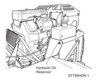
Figure 7-2. Hydraulic Oil Reservoir
