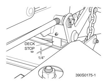
Figure 6-8. Cutter Deck Stop
