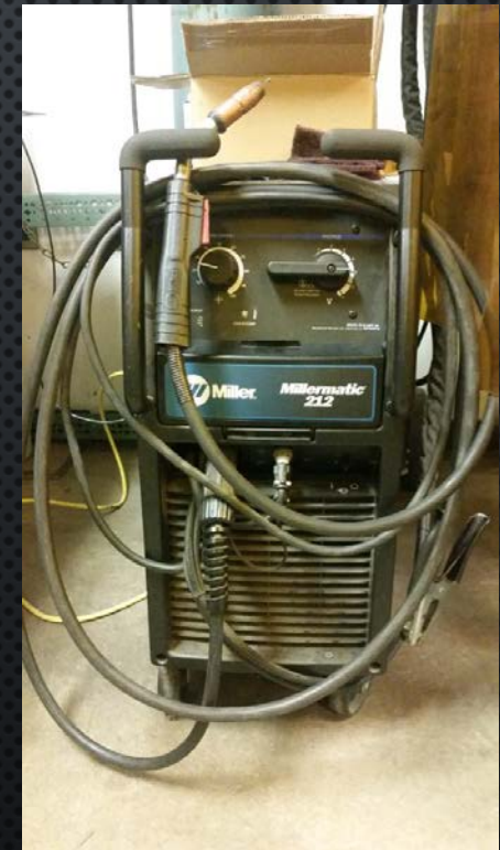
Miller Millermatic 212 M.I.G. Welder with Spoolmate3035 Spool Gun for Aluminum Welding
