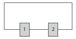
The total impedance of the circuit is the sum of the impedance of elements 1 and 2. Element 1 has a voltage of 25 volts and a current of 1 milliampere. Element 2 has a voltage of 20 volts and a current of 1.5 milliamperes. What is the total impedance of the circuit?
