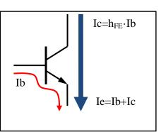
The gain ( $h_{FE}$ ) is the amount by which the transistor amplifies current. Usual values are around 100.
