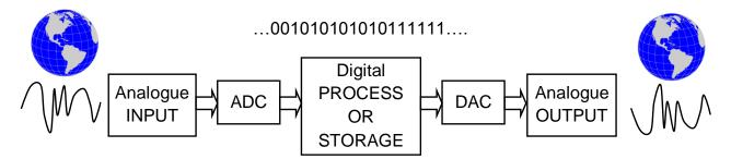
For example, we can get \_\_\_\_\_\_ with a microphone and analogue electronics. Then an ADC converts this signal to digital \_\_\_\_\_\_. This data can be \_\_\_\_\_\_ and stored in a digital format, such as \_\_\_\_\_\_.
