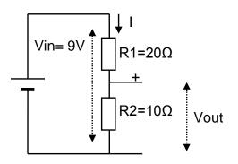
5b When one of the resistors is a special resistor the circuit is a sensor. Predict how light changes will affect Vout.
