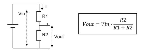
Potential dividers are used, for example, with LDRs in circuits which detect changes in light.
