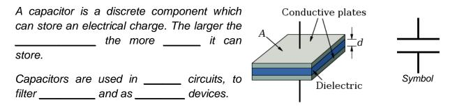
6b The unit of capacitance is the Farad. As this is a large amount, these submultiples are used:
