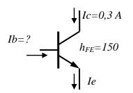
**12C** As with diodes, a voltage of 0.7V is necessary across the base-emitter to activate the transistor. In this circuit you can see the formula to calculate the current into the base. Then you can calculate the current into the collector.
