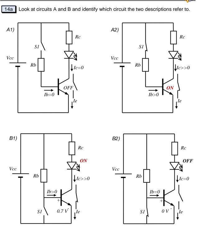
Circuit \_\_\_\_\_: When the switch is ON a current passes through the resistor into the base of the transistor. Then the transistor allows collector current to flow and the LED comes on.
