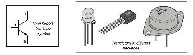
When a small \_\_\_\_\_\_ flows through the baseemitter circuit, a much larger current flows through the collector-emitter \_\_\_\_\_.
