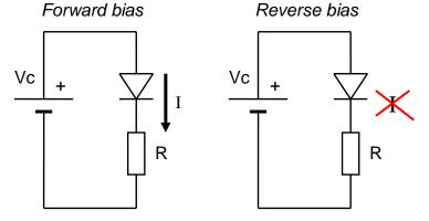
A diode is a semiconductor device that allows current to flow in one direction. It can be used for protection, to block signals, to change AC to DC, etc.
