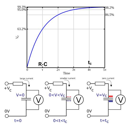
a) What % of the final voltage does the capacitor reach after  $\tau$ ? And after  $4\tau$ ?
