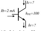
$Ic = h_{FE} \cdot Ib = 100 \cdot 2mA = 200 \ mA = 0.2 \ A$  $Ie = Ib + Ic = 2 + 200 = 202 \ mA = 0.202 \ A$
