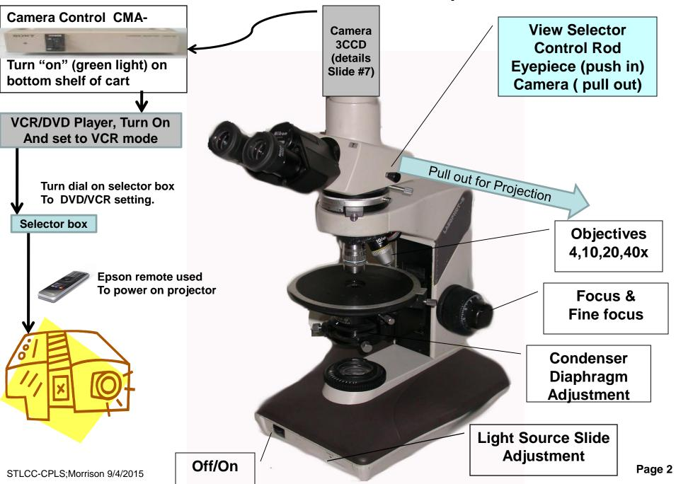
Microscopy: SM244 & SM245 Projecting the Microscope to Screen
