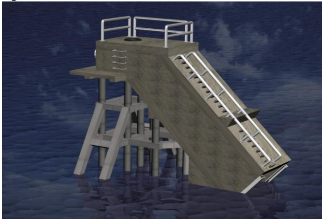
Gambar 3.4 Prototipe Sistem Oscillating Water Colum ( OWC ) [3]
