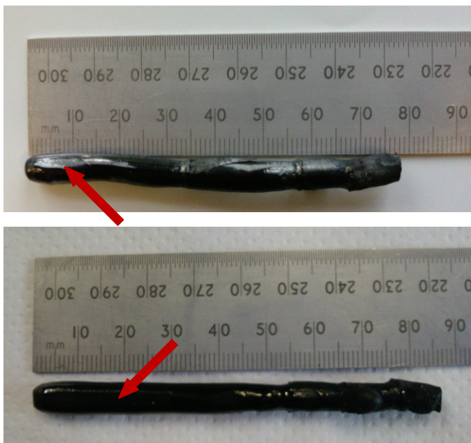
Fig.3.1: Single crystal boules (a) \text{CO}_2/\text{CO}=3 , (b) \text{CO}_2/\text{CO}=5 . Red arrows mark the facets formed during cooling.
