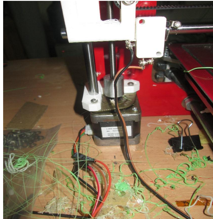
Fig-35: X-end motor & belt drive, bushing,
