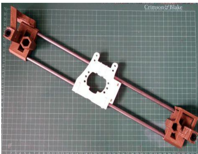
Fig-29: Assembled X-axis with two smooth rods, the X-end idler and X-end motor printed parts and the printed X-carriage:
