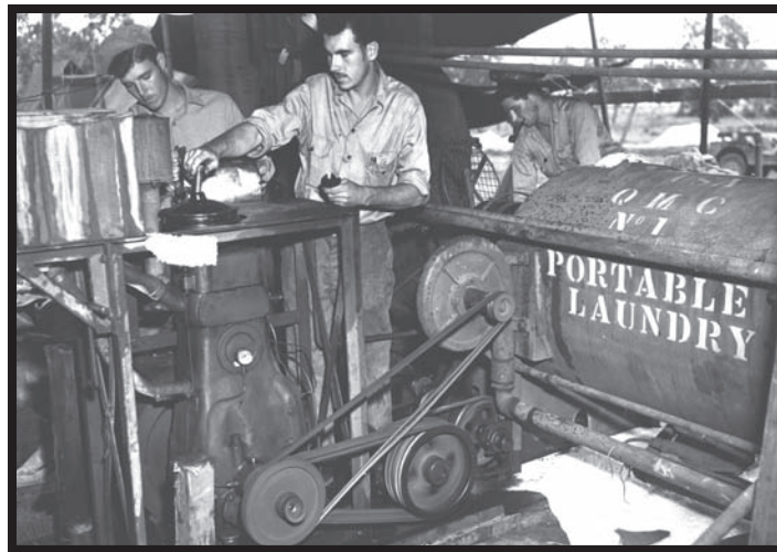
The QM's portable laundry diesel engine somewhere on New Guinea. 1943, (National Archives.)
