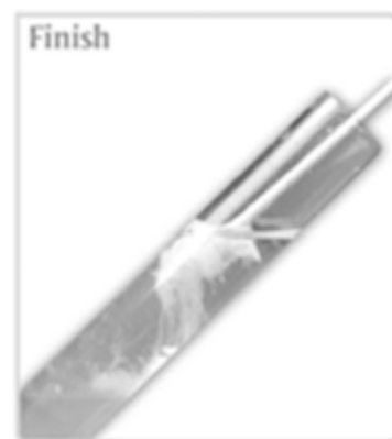
Twisting the DNA out of the test tube using a glass rod
