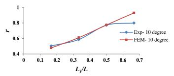
Fig. 12. Variation of natural frequency ratio with crack location ratio.
