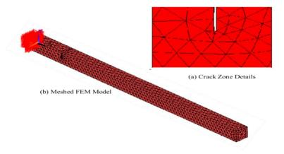
Fig. 3. A cracked beam finite element modelling.
