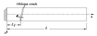
(b) Cantilever Beam with Oblique Crack
