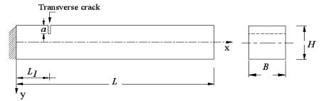
(a) Cantilever Beam with Transverse Crack
