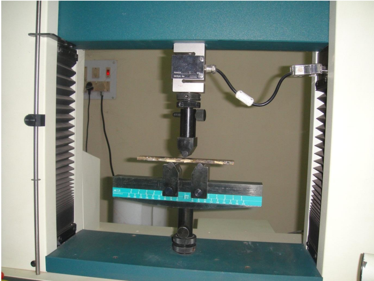
FIG(5.2) UTM machine Sample loaded condition for Flexural testing.
