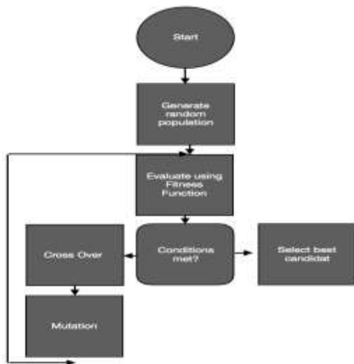
Figure 2: Flow chart of the simple genetic algorithm which correlates with the extraction of clear information, removing malfunctioned signals/information from the transmitted information
