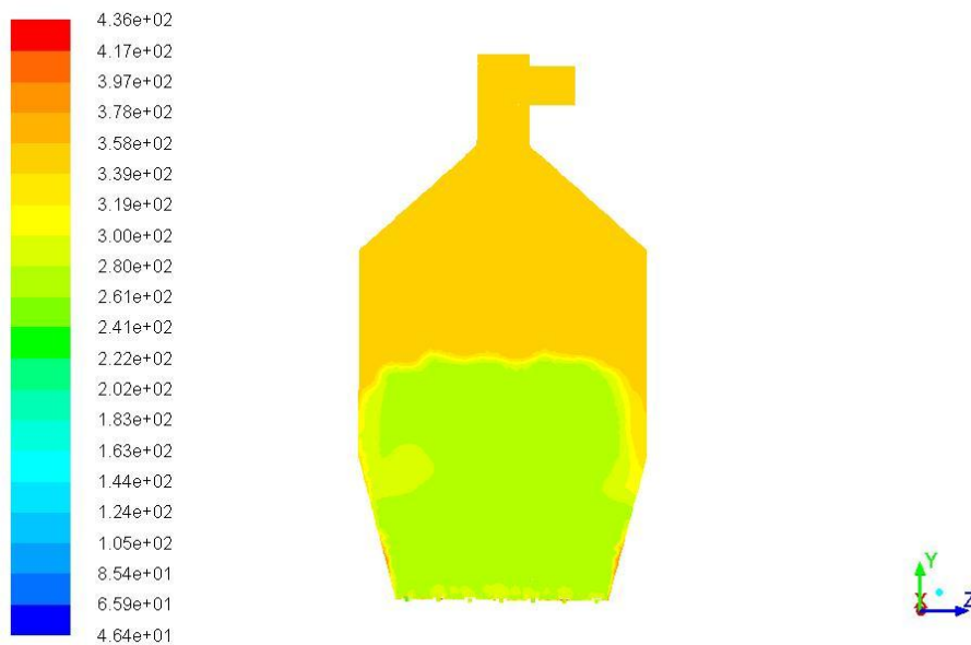
Figure 14: Contour of solid phase (Sand) temperature inside dryer
