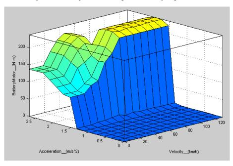
Figure 20. Electric Motor Torque vs. Acceleration and Velocity
