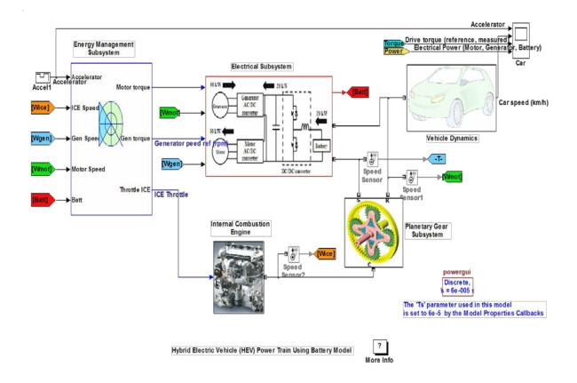
Figure 4. Simulation Model in SIMULINK for Hybrid Electric Vehicle Power Train Model
