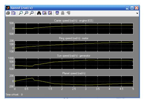
Figure 15. Planetary Gear Subsystem result
