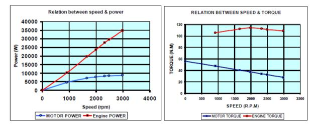
Figure 3. performance for hybrid and IC engine
