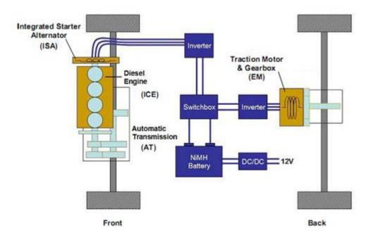
Figure 1. Ohio State Challenge X Vehicle Architecture [5]
