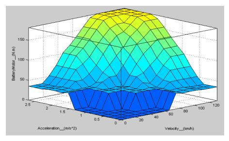
Figure 21. Hill shape: Torque increases with velocity and acceleration
