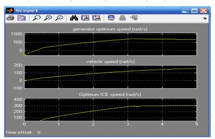
Figure 11. generator optimum speed, Vehicle speed and Optimum ICE speed (rad/s)
