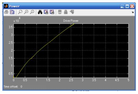
Figure 10. Relationship between drive power and time at Speed range 0:60Km/h
