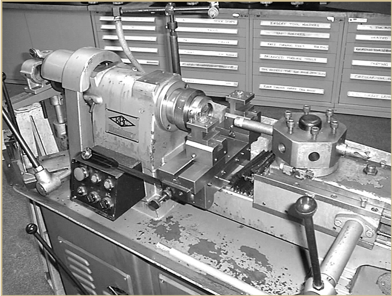
FIGURE 43— This is an example of a conventional lathe with a turret that can hold multiple cutting tools. The operator manually rotates the turret after each cutting operation.
