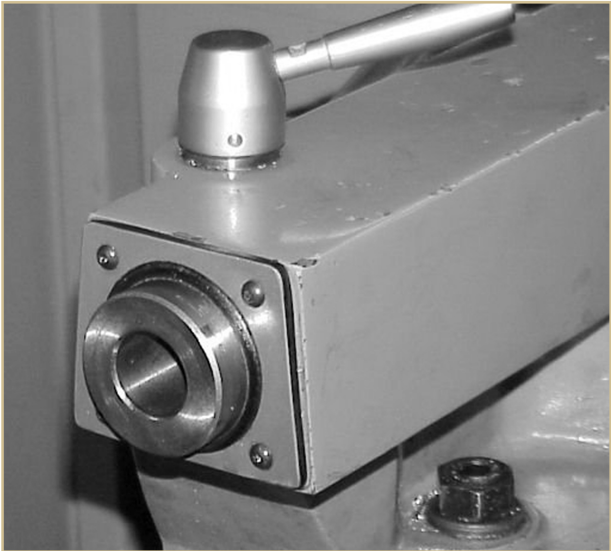
FIGURE 10 —Collets and tapered cutting tools can be inserted into this lathe tailstock, which has a taper that matches the one found on the cutting tool or toolholder.
