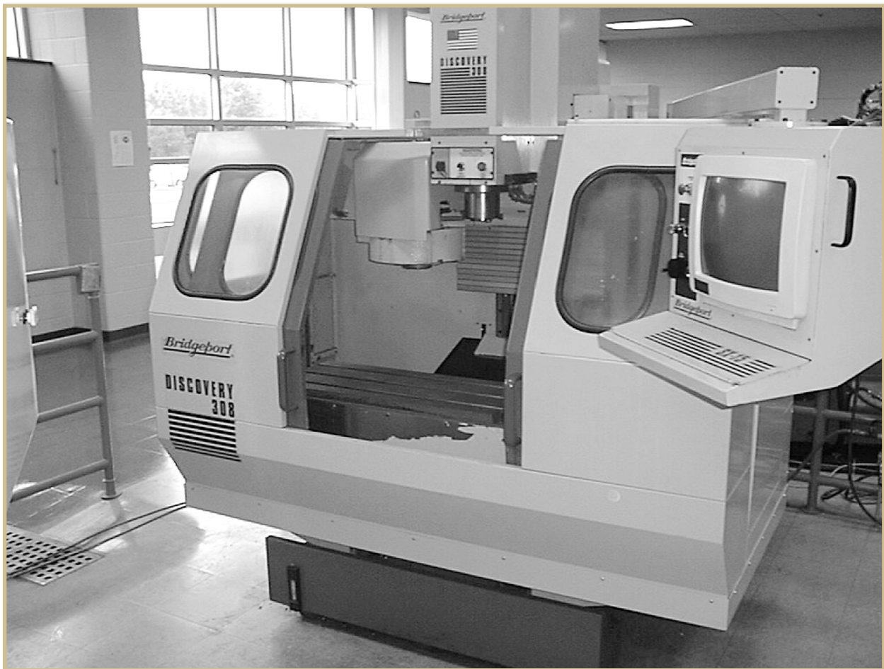
FIGURE 2—A modern machining center includes a computer to control the machining process. The doors lock in the closed position during machining to ensure operator safety.
