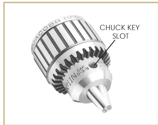
FIGURE 34—Adjustable collets or drill chucks are available for general-purpose use in a lathe or drill press. They aren't used for precision applications due to the chance of poor concentricity of the cutting tools when placed in the collet. (Courtesy of DoAll Company, Des Plaines, IL)
