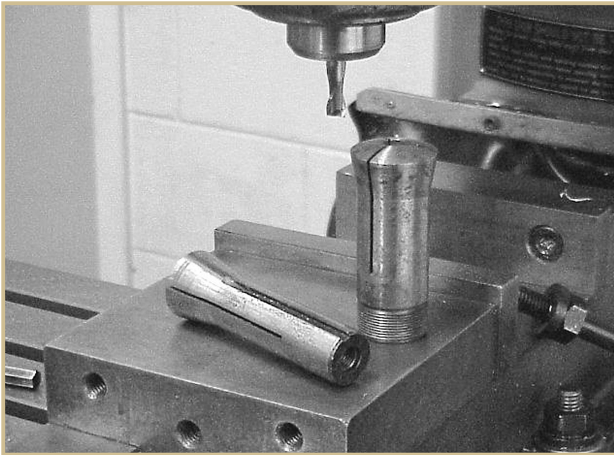
FIGURE 9 —These spring-type collets can be used in both lathes and milling machines. The precision spring fingers provide good concentricity with cutting tool changes.
