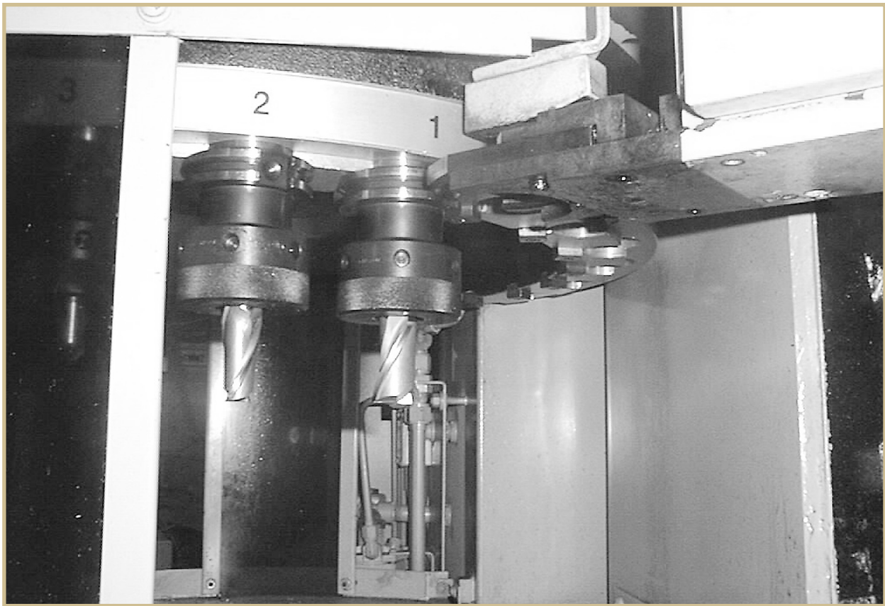
FIGURE 44 —Many machine cutters have toolholders loaded in a magazine to allow a tooling change controlled by a computer. Tool changes can take place in seconds without operator intervention.
