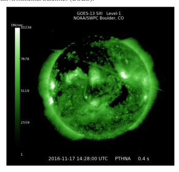
Figure 3–10.—An x-ray image of the Sun taken in 2016, from the GOES-13 solar xray imager (SXI). Various exposure settings are captured throughout a sequence of images taken each minute. This particular image (Level-1) allows a better look at coronal structure; as well as some examination of active regions and flares.
