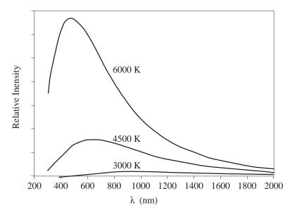
Figure 3–9.—Schematic blackbody radiation curves at three temperatures. The wavelength of maximum intensity varies inversely with the absolute temperature as in the formula
