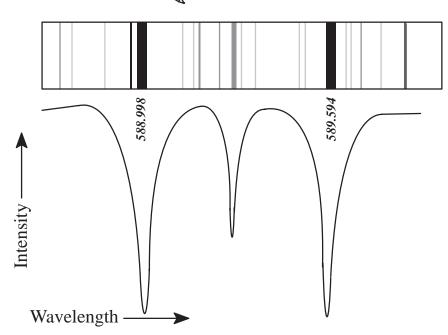
Figure 3–5.—Schematic of Sodium absorption from a Solar white-light spectrum. Top: The two dark absorption lines with wavelengths of 589.0 and 589.6 nanometers are produced by sodium atoms absorbing at these wavelengths. Fraunhofer observed these two lines as one, which he named the "D" line. Bottom: The same spectrum as seen on a graph of intensity versus wavelength. Each dark line appears as a drop in intensity, where light is subtracted from the continuous spectrum.
