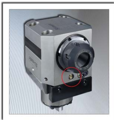
1,450 PSI high pressure axial internal coolant tool with switch on front of tool for directing coolant flow between internal coolant and external coolant.
