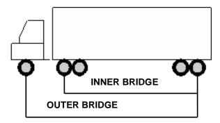
Maximum gross vehicle weight with maximum tandem axle weight of 44, 000 lbs.
