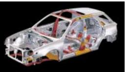
Careful computer analysis and design provides a structure that's stronger and more rigid than the previous Impreza. Front and rear crumple zones help manage impact energy by compressing at a controlled rate.
