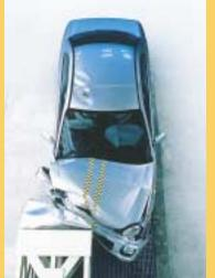
Ring-Shaped Reinforcement Frames in the front, center and rear of the body structure disperse impact energy around the passenger compartment, offering added protection for occupants. The center ring connects the center pillar with the lateral roof and floor supports for increased side-impact protection. In addition, a specially designed front sub-frame increases energy absorption in offset frontal collisions.
