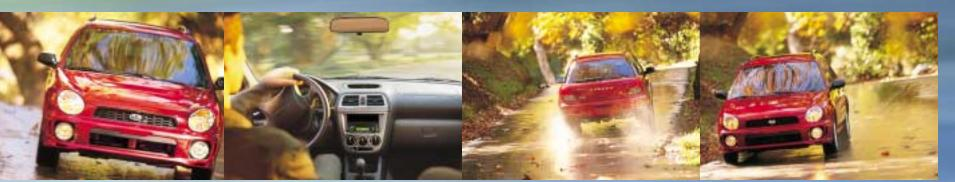
Going into a corner, rear-wheel drive cars tend to oversteer. The rear wheels can break loose, sending the car into a spin. Subaru AWD tracks smoothly through the curve, entering with the right amount of power to the front wheels. Coming out of a corner, a front-wheel drive car tends to understeer, or plow toward the outside of a curve when accelerating. With AWD, the Subaru Impreza exits a curve with the right amount of power to the rear wheels.
