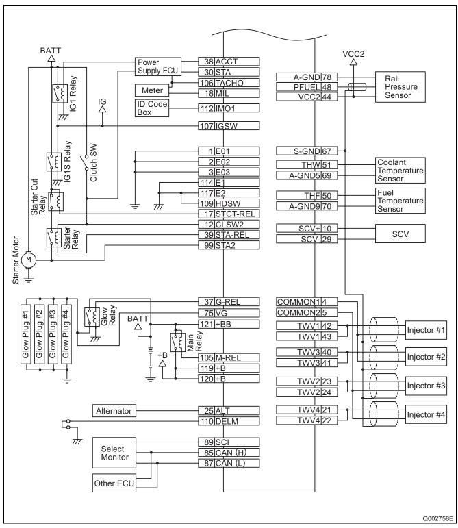
Engine ECU External Wiring Diagram (2)
