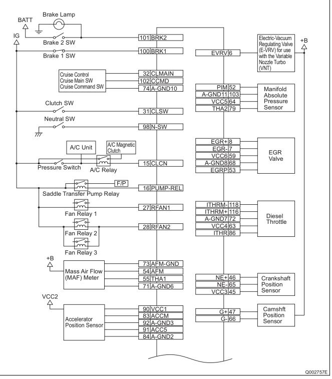
Engine ECU External Wiring Diagram (1)
