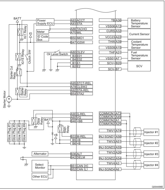
Engine ECU External Wiring Diagram (2)
