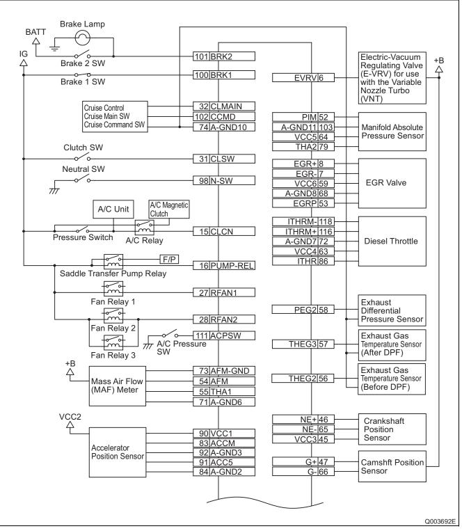
Engine ECU External Wiring Diagram (1)
