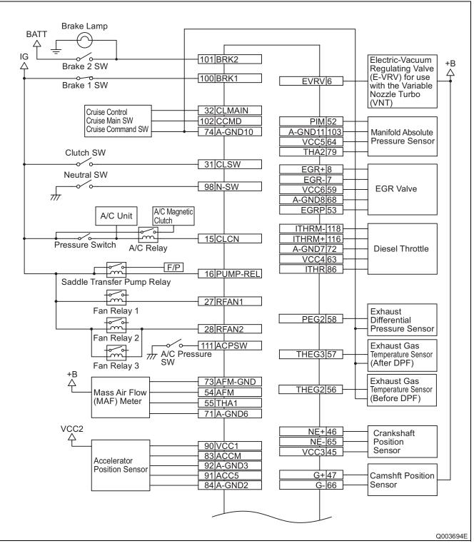
Engine ECU External Wiring Diagram (1)
