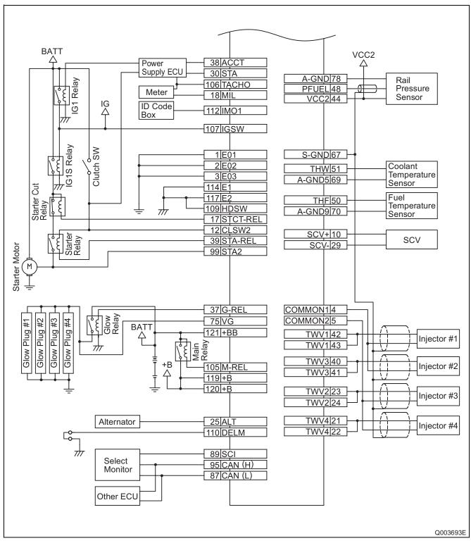
Engine ECU External Wiring Diagram (2)
