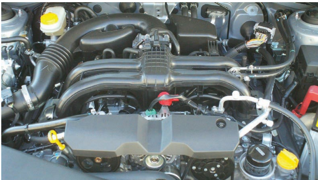
The new Subaru FB horizontally opposed 4-cam 4-cylinder replaces the EJ that dates back to 1989.
