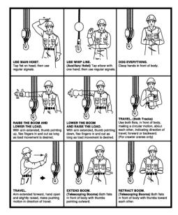
Hand signals should be used only when the operator has a clear view of the signaler. The international hand signals for hoisting shall be used.
