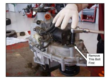
7. Remove the three (3) bolts around the head area of the shift motor.
