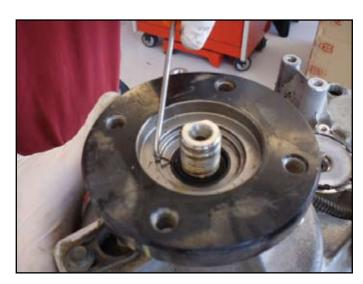
11. Remove the output shaft flange from the transfer case. Remove rear damper weight if necessary.
