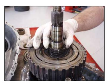
24. Install the cam with three (3) steel balls.
