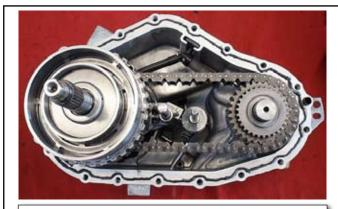
Do not use RTV around bolt holes, apply as shown. Use a 2mm drill bit to pierce hole in RTV Tube.
