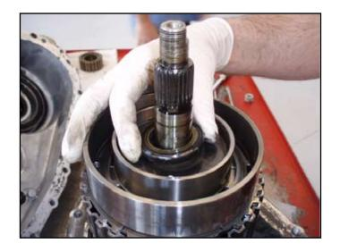
15. Remove the cam coil housing cover.
