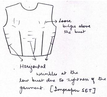
The problem can be rectified by opening the dart and relocating the dart by marking the bust point lower than before.
