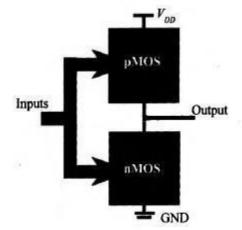
Fig. 5.1 Standard configuration of a CMOS complementary gate.
