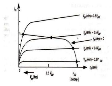
From the graph it is clear that as Vin(=Vgs p.d. transistor) exceeds the Pulldown threshold voltage current begins to flow. The output voltage Vout thus decreases and the subsequent increases in Vin will cause the Pull down transistor to come out of saturation and become resistive.
