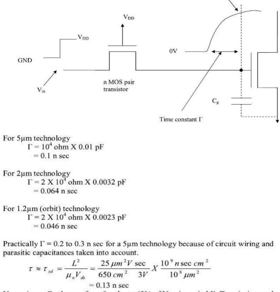
$V_{ds}$  varies as  $C_g$  charges from 0 volts to 63% of  $V_{DD}$  in period  $\Gamma$ . Transit time and time constant  $\Gamma$  can be used inter changeably.
