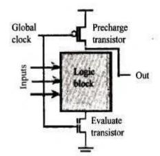
Basic Structure of a dynamic CMOS gate
