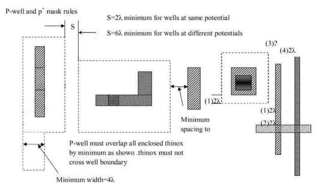
The CMOS rules are designed based on the extensions of the Mead and Conway concepts and also by excluding the butting and buried contacts the new rules for CMOS design are formed. These rules for CMOS design are implemented in the above diagrams.
