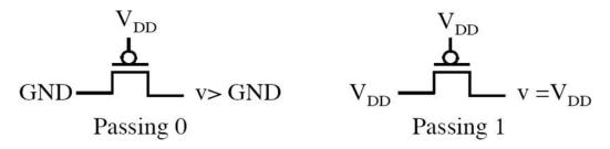
This is the reason that N-Channel transistors are used in the pull-down network and P-Channel in the pull-up network of a CMOS gate. Otherwise the noise margin would be significantly reduced.
