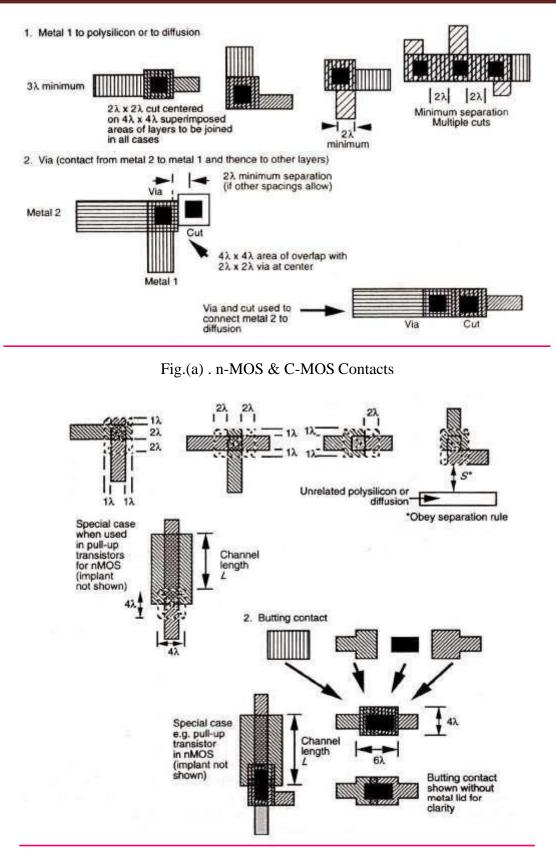
Fig.(b). Contacts poly-silicon to diffusion
