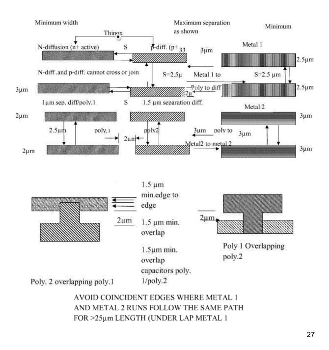
Design rules for wires (interconnects) (orbit 2µm CMOS)
