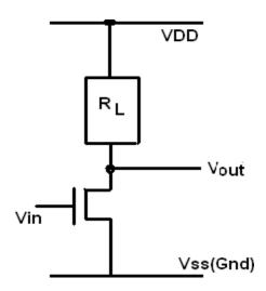
**nMOS depletion mode transistor pull-up :** This arrangement consists of a depletion mode transistor as pull-up. The arrangement and the transfer characteristic are shown below. In this type of arrangement we observe
