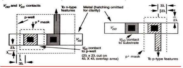
In the diagram above each of the arrangements can be merged into single split contacts.
