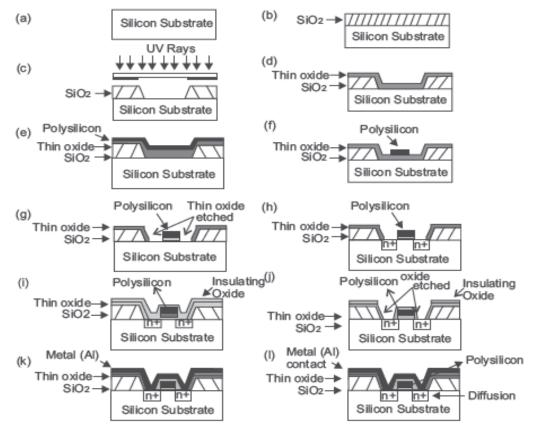
Figure 1.9: Fabrication Process of NMOS Device
