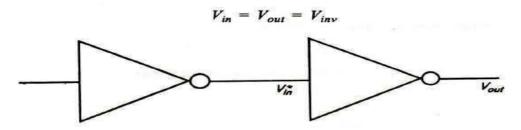
Fig.(a).Inverter driven by another inverter.
