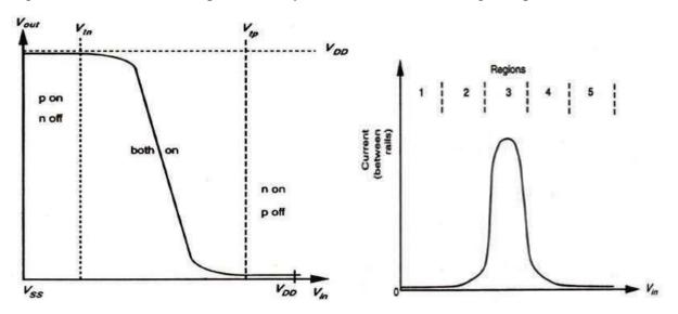
Hence the output voltage is logic 1. In region 5,  $V_{in} = logic 1$  and the n-transistor is fully on while the p-transistor is fully off. So, no current flows and logic 0 appears at the output.
