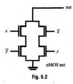
2. Implement the pMOS net as a dual topology to the nMOS net. The pMOS transistors driven by  $\bar{x}$  and y are connected in parallel, as are the devices driven by x and  $\bar{y}$  (Fig. 5.3). These transistor groups are connected in series, since they are parallel connected in the nMOS net. The *out* node now implements  $\bar{F}$ .
