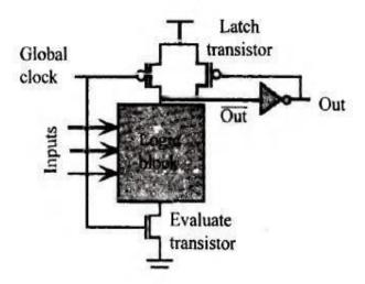
Fig. 5.12 Domino CMOS logic gate with feedback transistor.
