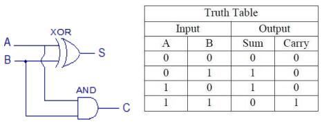
The carry-out is equivalent to a carry-in to the next more significant column of a multibit adder, so it can be described as having double the weight of the other bits. If multiple adders are to be cascaded, each must be able to receive the carry-in. Such a full adder has a third input called C or Cin.
