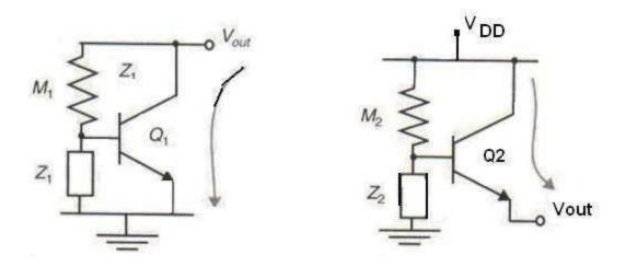
The impedances Z2 and Z1 are used to bias the base-emitter junction of the bipolar transistor and to ensure that base charge is removed when the transistors turn off. For example when the input voltage makes a high-to-low transition, M1 turns off first. To turn off Q1, the base charge must be removed, which can be achieved by Z1.With this effect, transition time reduces. However,
