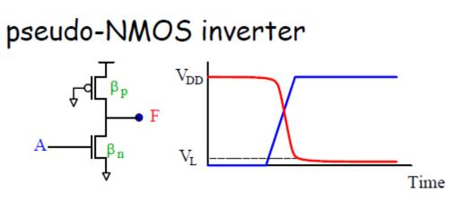
The inverter that uses a p-device pull-up or loads that has its gate permanently ground. An n-device pull-down or driver is driven with the input signal. This roughly equivalent to use of a depletion load is **NMOS** technology and is thus called '**Pseudo-NMOS**'. The circuit is used in a variety of CMOS logic circuits.
