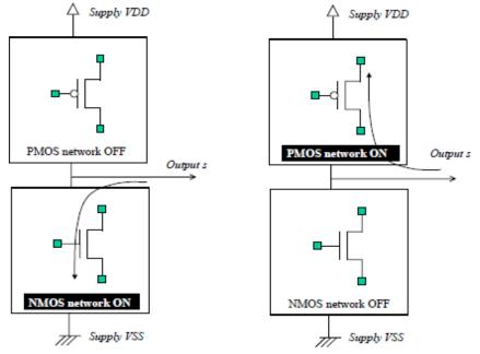
Fig. 6-6. General structure of a CMOS basic gate
