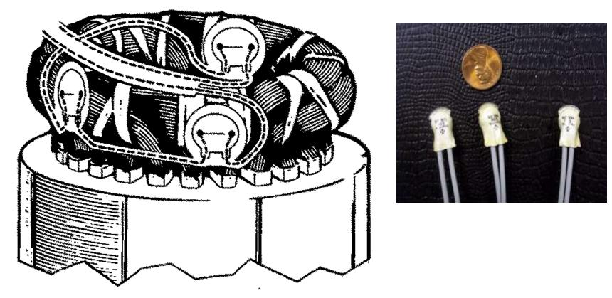
Three (3) Switches Wired In Series, Placed In The Stator End Turns
