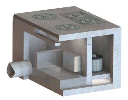
**Manhole:** The Manhole PerkFilter contains from one to eleven cartridge stacks and is provided in a concrete manhole structure that can range from 48" to 96" in diameter. Stormwater is typically delivered to the Manhole PerkFilter through an inlet pipe connection. The Manhole PerkFilter includes a high-flow bypass that routes peak flows around the treatment chamber to discharge.
