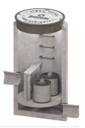
**Vault:** The standard Vault PerkFilter can contain up to 31 cartridge stacks and is provided in a precast concrete vault ranging in size from 4' x 4' up to 8' x 18'. Stormwater is typically delivered to the Vault PerkFilter through an inlet pipe connection. The Vault PerkFilter includes a high-flow bypass that routes peak flows around the treatment chamber to discharge.
