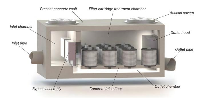
Figure 1. Schematic of the PerkFilter System
