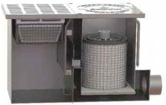
These systems have a maximum depth of 5 feet from the rim to the invert of the outlet pipe. The minimum depth is dictated by the cartridge stack height. The catch basin configuration can also accommodate an inlet pipe if needed, and includes a high-flow bypass that routes peak flows around the treatment chamber to discharge.
