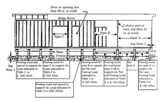
Notes: 1. Bottom of footings must be below the frost line depth, unless designed for placement above the frost line. (See §3285.312(b)).
