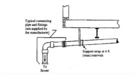
Figure A to § 3285.904 - Connection to Site Sewer.
