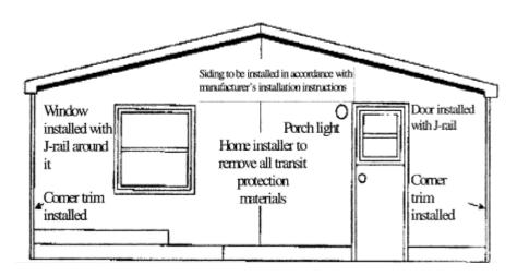
Notes: 1. Multi-section homes with horizontal-lap siding can be shipped with no siding on the front and rear end walls.
