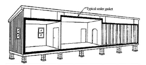
Figure B to § 3285.801 Mate-Line Gasket.
