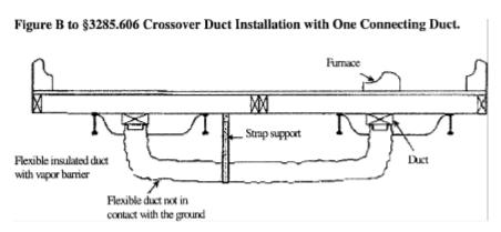
Notes: 1. This system is typically used when a crossover duct has not been built into the floor and the furnace is situated directly over the main duct in one section of the home. A single flexible duct is then used to connect the two sections to each other.
