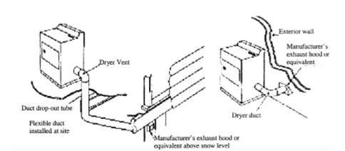
Figure A to § 3285.503 Dryer Exhaust System.
