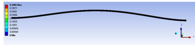
Figure.4: Maximum Deformation (50m free span)
