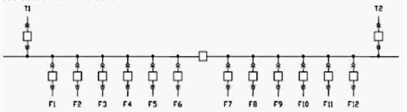
Figure 1: Single Bus scheme with Bus Section Breaker
