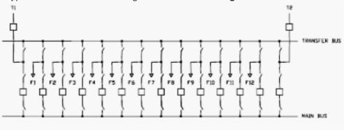
A typical transfer busbar arrangement is shown in *Figure 6*.
