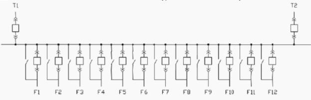
Figure 2: Single Bus scheme with Bypass Isolator
