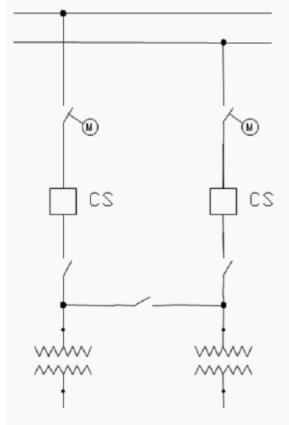
Figure 10: Double feed Scheme
