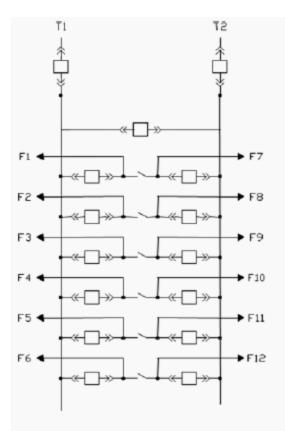
Figure 3: Single Bus scheme with Bypass Switch between Two adjacent Bays
