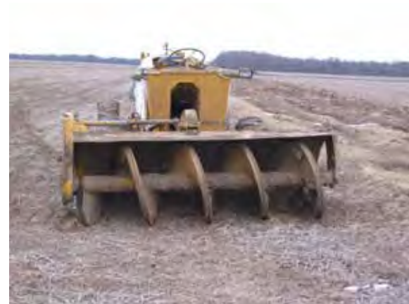
Machine designed for backfilling. It uses a auger to move the excavated material.
