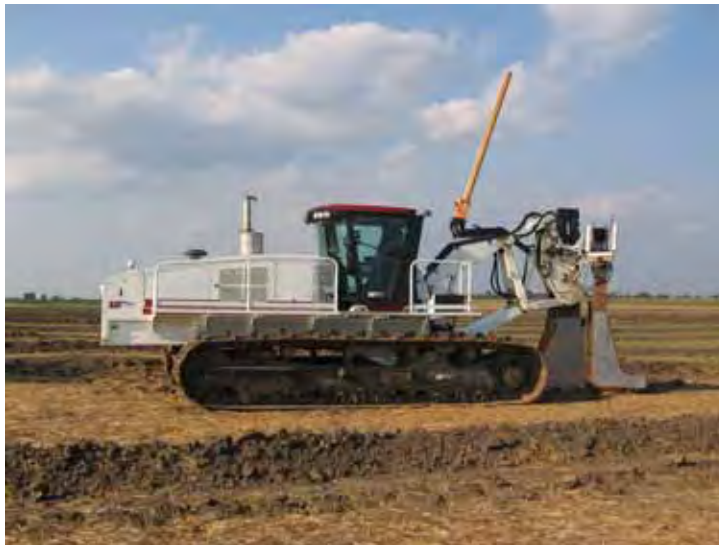
Trenchless type tile machine.
