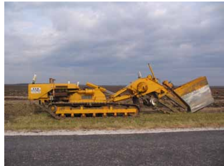
Trencher type tile machine. This machine uses a chain with “teeth” to excavate the trench.
