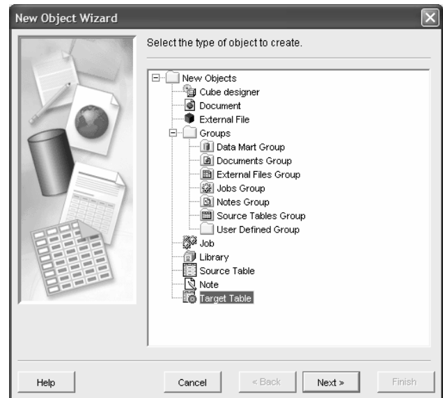
Figure 12. The New Object wizard is used to add a target table definition to a project. Other object types can be added in the same way.
