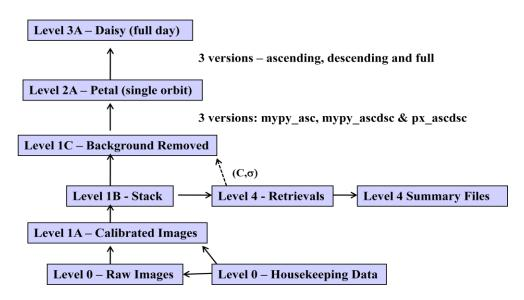
**Figure 1.** Flow chart illustrating the data processing flow and definition of CIPS data levels for all V3.X data versions.
