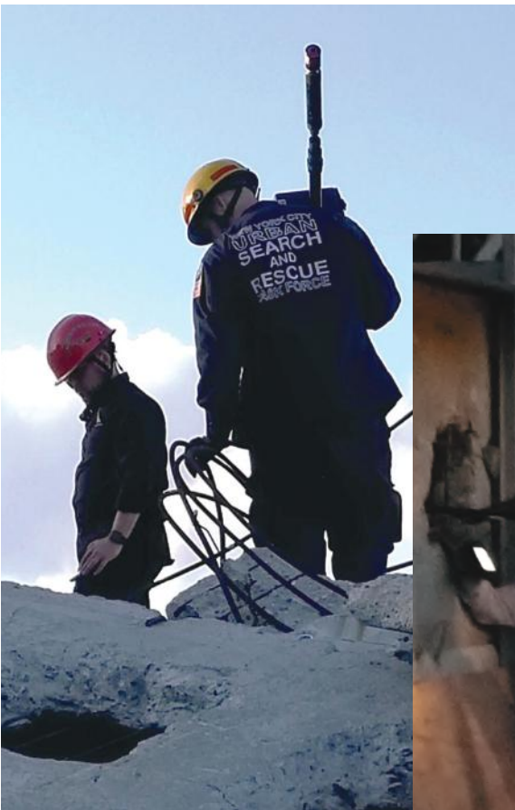
USAR members utilizing the advanced articulating-tipped camera (above and at right) to probe through tight spaces and give them a 360 degree view inside the rubble.
