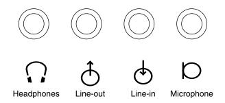
FIGURE B-11 Audio Connector Configuration
