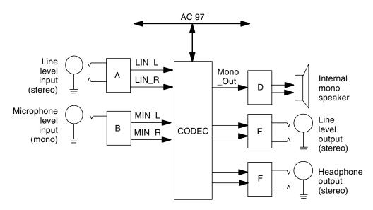
FIGURE C-6 Audio Circuit Functional Block Diagram
