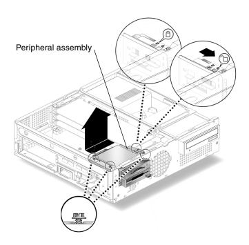
FIGURE 7-1 Removing and Replacing the Peripheral Assembly
