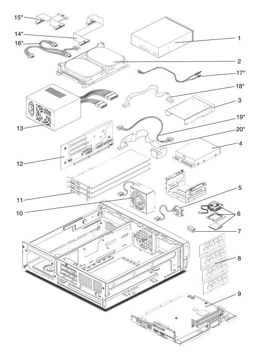
FIGURE 1-4 Sun Blade 150 System Replaceable Parts
