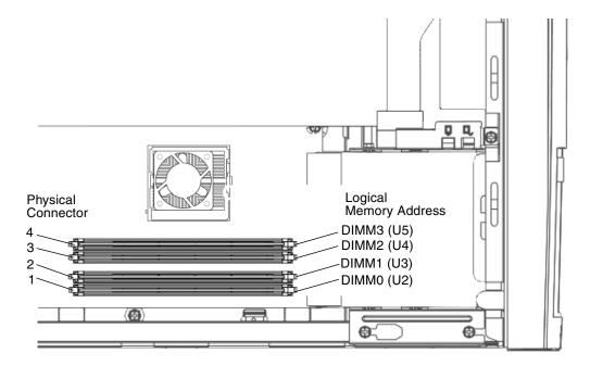
FIGURE 8-4 DIMM Installation Order
