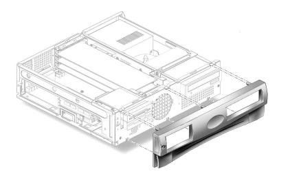
FIGURE 6-7 Removing the Front Bezel
