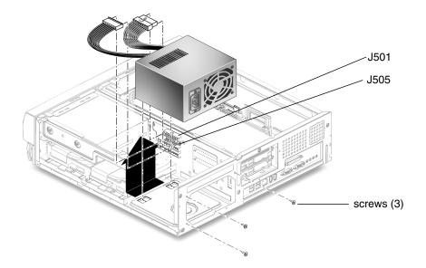
FIGURE 6-1 Removing and Replacing the Power Supply
