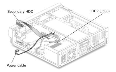
FIGURE 7-6 Secondary Hard Drive Cabling Configuration
