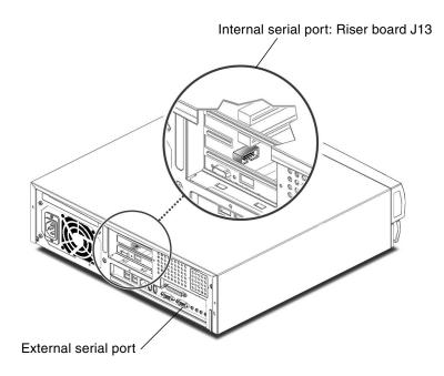
FIGURE B-8 Accessing the Second Serial Port Through a PCI Card Slot
