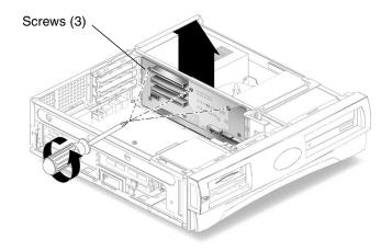
FIGURE 8-9 Removing and Replacing the Riser Board
