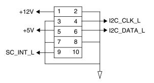
FIGURE C-8 Smart Card Interface Header
