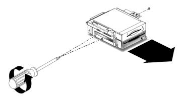
FIGURE 7-2 Removing the Diskette Drive
