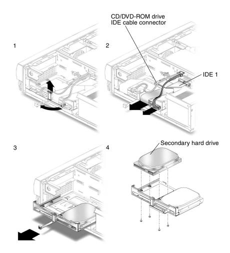
FIGURE 7-5 Installing a Secondary Hard Drive
