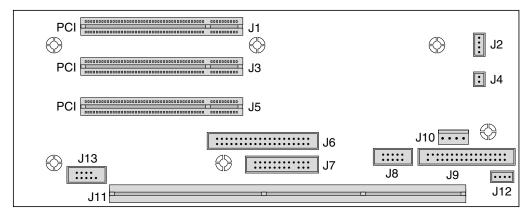
FIGURE C-3 Riser Board Layout Diagram, Side 1
