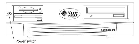
FIGURE 9-2 System Power Switch
