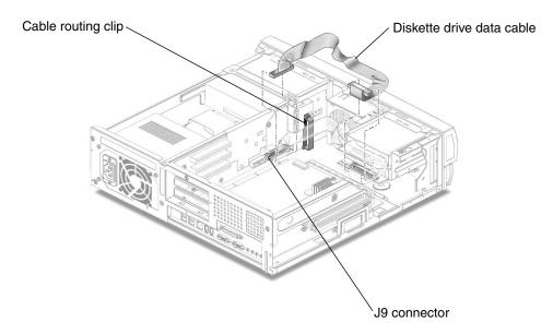
FIGURE 6-2 Removing and Replacing the Diskette Drive Data Cable Assembly
