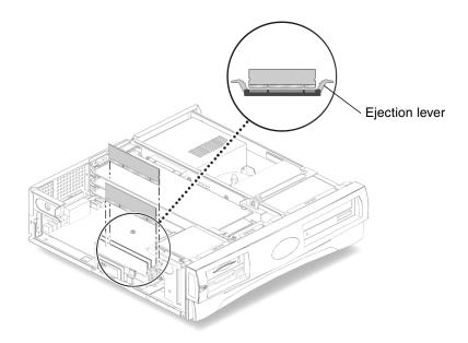
FIGURE 8-5 Removing and Replacing a DIMM
