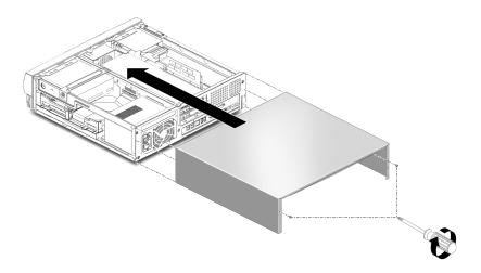
FIGURE 9-1 Replacing the System Cover
