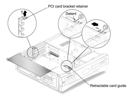
FIGURE 8-6 Removing and Replacing a PCI Card
