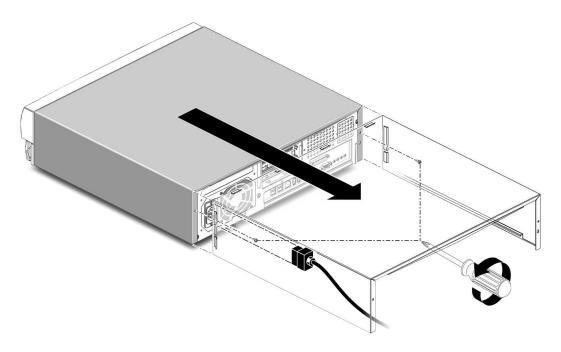
FIGURE 5-2 Removing the System Cover
