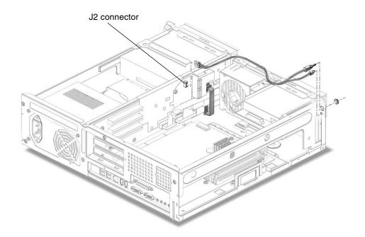
FIGURE 6-8 Removing and Replacing the Power Switch/LED Assembly
