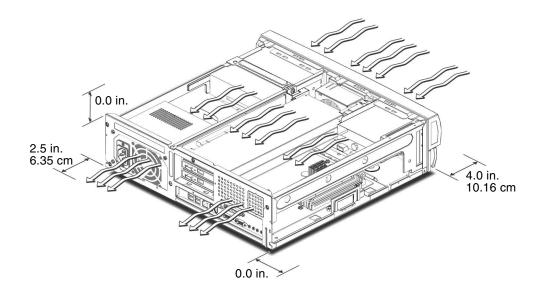
FIGURE A-1 Minimum Clearance for System Cooling
