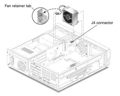
FIGURE 6-10 Removing and Replacing the Fan Assembly
