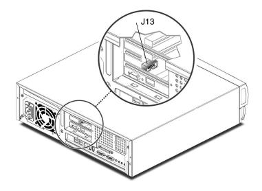
FIGURE C-5 External and Internal Serial Ports
