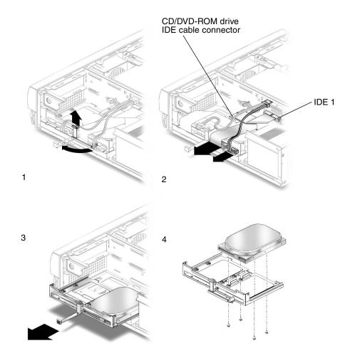
FIGURE 7-4 Removing and Replacing a Primary Hard Drive
