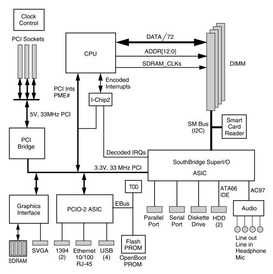
FIGURE C-1 Sun Blade 150 System Functional Block Diagram
