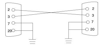
FIGURE 3-1 Setting Up a TIP Connection
