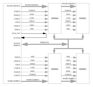
FIGURE C-11 Sun Blade 150 Memory Block Diagram
