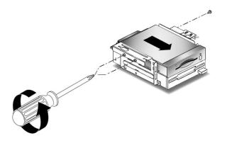
FIGURE 7-3 Removing and Replacing the Smart Card Reader
