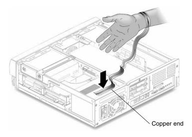
FIGURE 5-3 Attaching the Wrist Strap to the Chassis
