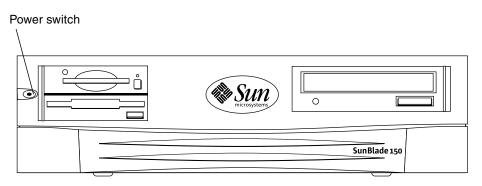
FIGURE 5-1 Front Panel Power Switch
