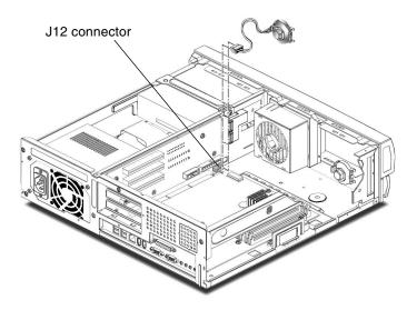
FIGURE 6-9 Removing and Replacing the Speaker Assembly
