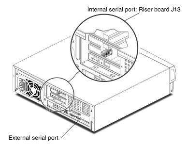
FIGURE A-3 External and Internal Serial Ports
