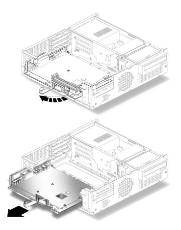
FIGURE 8-7 Removing and Replacing the Motherboard
