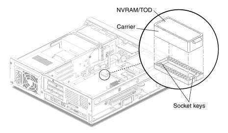
FIGURE 8-3 Removing and Replacing the NVRAM/TOD
