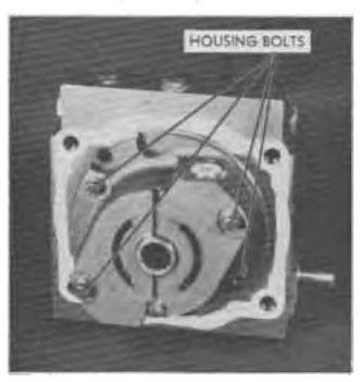
FIG. 63. Charge Pump Housing
