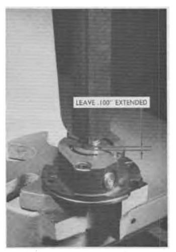
FIG. 54. Needle Bearing Installation
