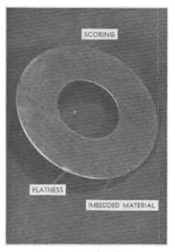
FIG. 45. Inspect Thrust Plates
