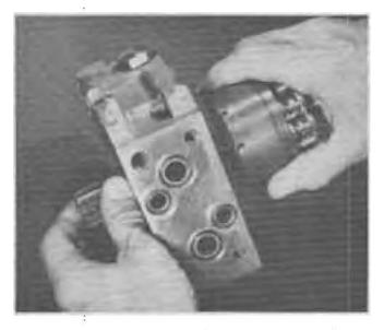
FIG. 85. Install Piston-Cylinder Block Assembly
