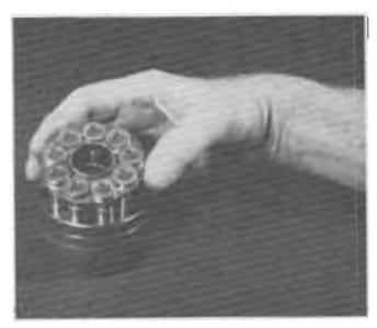
FIG. 42. Check Free Movement of Pistons
