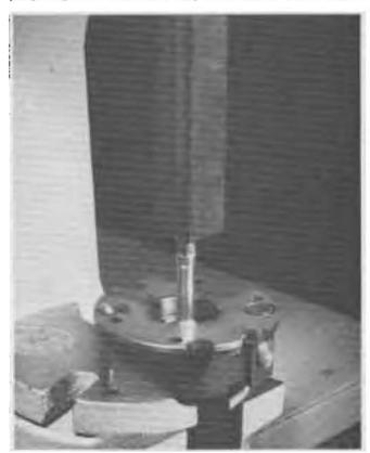
FIG. 53. Needle Bearing Removal
