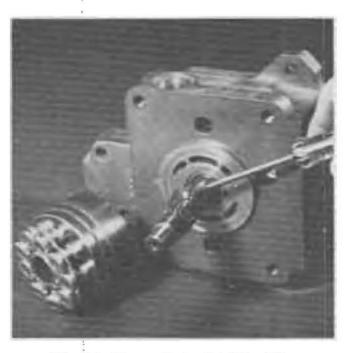
**FIG. 77.** Remove Spring Retaining Clip
