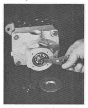
FIG. 71. Remove Snap Ring from Motor Shaft
