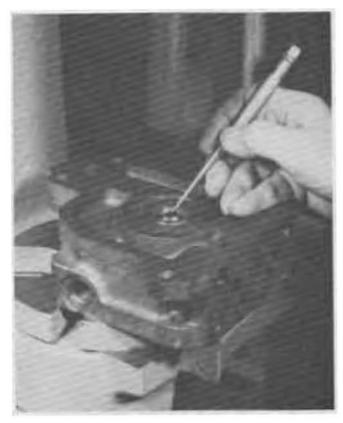
FIG. 79. Remove Seal Retainer "O" Ring
