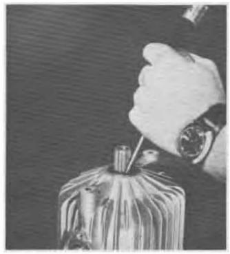
FIG. 55. Seal Removal
