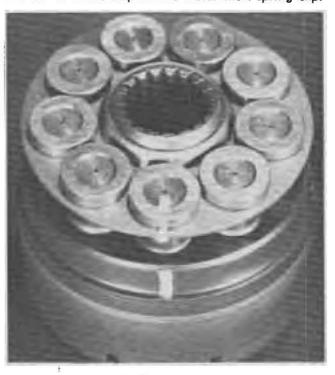
FIG. 88. Before removing Pitton, Mark both Piston and Cylinder Bore with Tape
