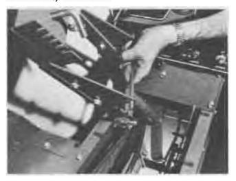
FIG. 34. Seat Pivot Installation
