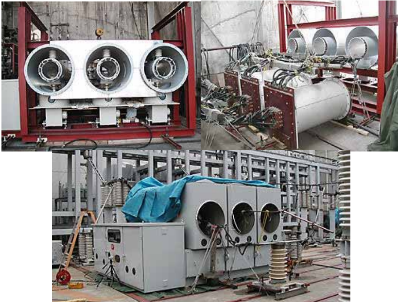
Gambar X. 20 Alternating Current Withstand Voltage Test
