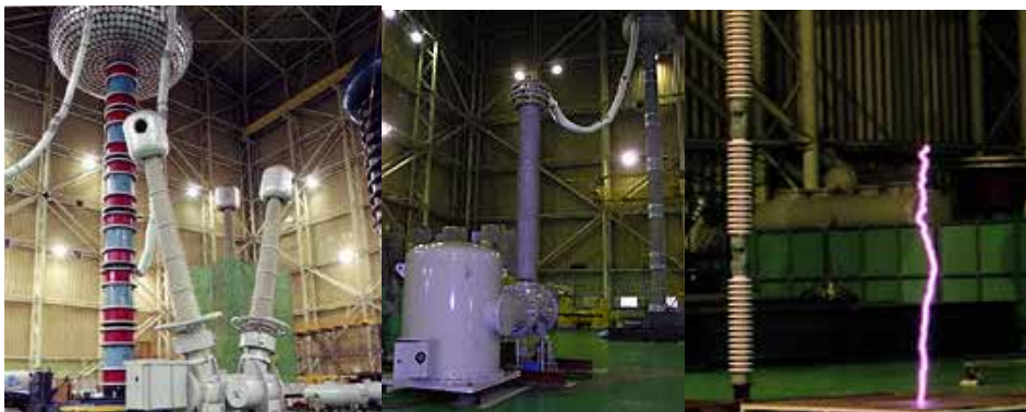
Gambar X.21 Internal Arc Test of Cubicle
