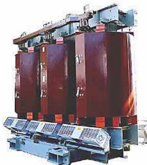
Gambar X. 17 Sheet-Winding (standard; aluminum optional; copper) 3-phase 50Hz 10,000kVA 22/6.6kV
