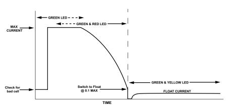
**Bulk Charge....** This is a high current state, selected by the maximum current setting (Fuse Jumper), and controlled by the battery's voltage. The charger will provide up to maximum current, limited by the circuit, the power supply voltage, and the battery's impedance and voltage.
