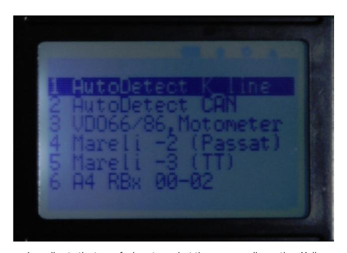
According to the type of odometer, select the corresponding option. Maily odometer is divided into K line and CAN line, but the K line and CAN have different manufacturers, different versions, different types of odometer. User can
