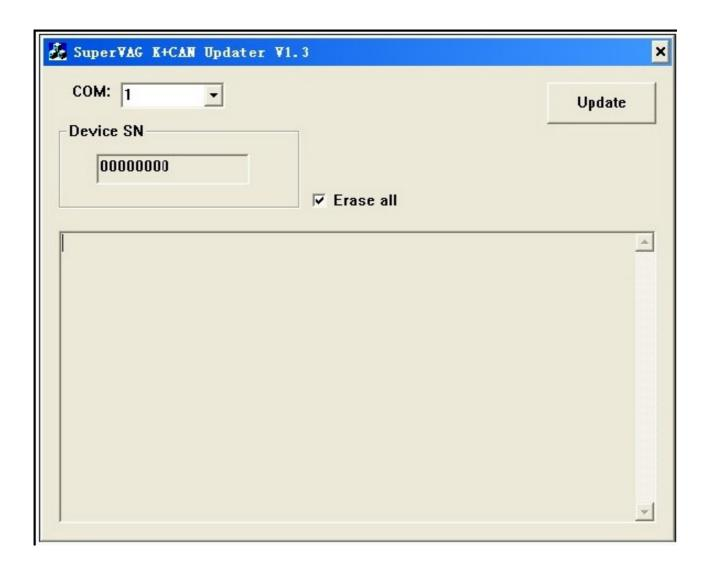
To choose the correct communication port, the communications port, you can set in operating system's "Device Manager"
