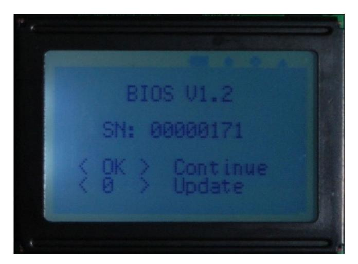
Input 0 in keyboard, when appear the following interface, it means the device has entered the state to upgrade.
