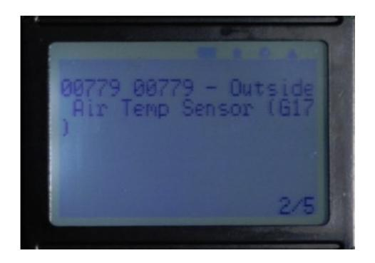
Press <O> keys to read the next fault code, and <P> key to read the last fault code, press BACK button to return to previous menu. Fault code also supports multi-language
