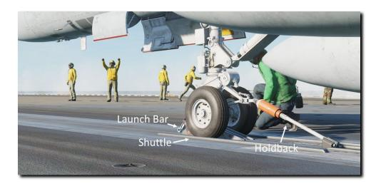
**5. Seat launch bar in shuttle.** When directed, raise the launch bar to seat it in the catapult shuttle. Note that the bar will not fully retract until it is clear of the shuttle after launch.
