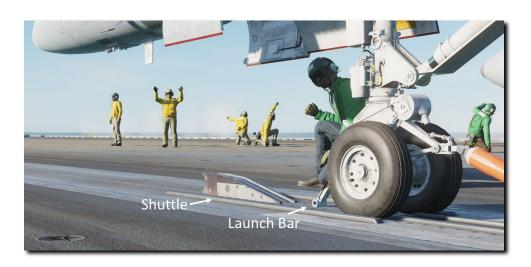
**4. Connect to catapult shuttle.** Following the Director's signals, taxi forward slowly to position the launch bar over the shuttle. Significant power, as much as 80-85% RPM, may be required. When the launch bar drops over the shuttle, the aircraft will be stopped as the holdback engages the catapult buffer. Reduce power to idle.
