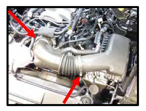
28. Remove the airbox bottom by removing the (1) bolt on the driver side inner fender (10mm socket).
