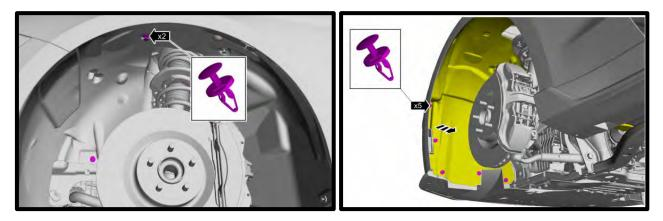
10. Remove the push pins from the (2 per side) push pins securing inner fender well to undertray.
