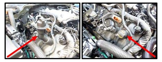
19. Remove the PCV purge line from the intake manifold and RH cam cover. One of these 90deg connectors will be reused.
