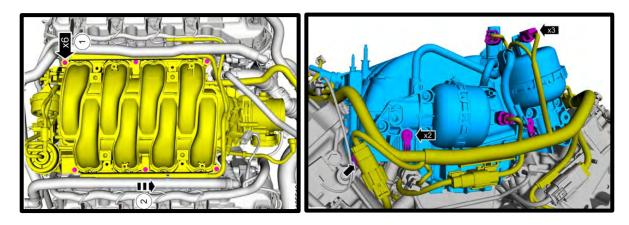
40. Clean the intake manifold to cylinder head surface using carb cleaner or acetone. Install tape over the exposed ports until manifold installation.
