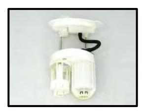
153. (Stage 2 and Up Systems) Remove the (3) locating tabs and smooth the pump receptacle to the diameter of the DW400 (46mm).
