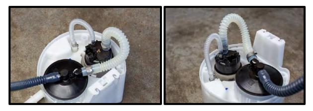
156. (Stage 2 and Up Systems) Install the new connector harness supplied with the DW kit, the additional static ground inserts into the slot on the assembly filter, the same as OE.
