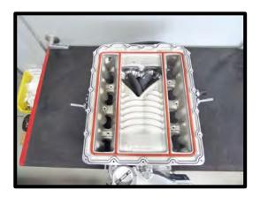
96. Install the (1) #2-230 internal bypass oring to the lid bypass passage. Use generous amount of grease to secure oring in place.
