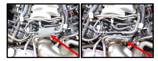
21. Disconnect and remove the brake aspirator lines from the inlet tube and intake manifold.
