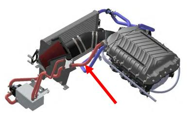
132. Install the supplied 5/8" ID x 21" hose to the driver side valve cover. Push until it clicks and locks into place. The other end will be installed in inlet tube later.
