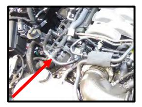
20. Pull apart the rubber shielding securing vacuum lines together.
