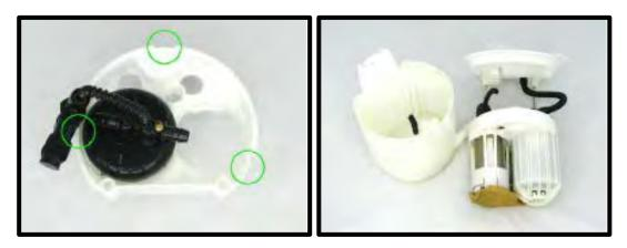
152. (Stage 2 and Up Systems) Carefully cut the larger pump outlet hose (3/8" ID) from the assembly filter and remove the OE pump.
