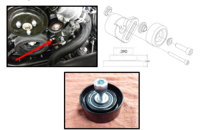
67. Remove the factory plastic smooth idler pulley from the engine. Replace with the supplied steel idler pulley. Use the factory fastener to secure. Torque to 18 lbs-ft with a 13mm socket. **NOTE:** Image shows proper direction of idler assembly.
