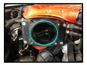
143. Install the stock throttle body using the (4) 6mm x 50mm FHSCS bolts using a 10mm socket.
