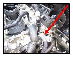
42. Remove the driver side heater tube from engine by removing the (1) bolt using an 8mm socket.
