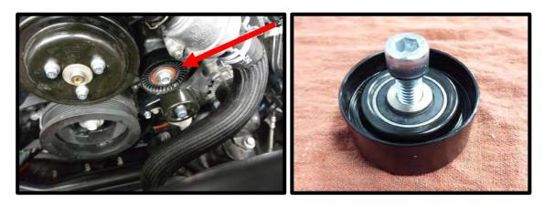
68. Assemble the spring-loaded tensioner by mounting the supplied spacer with the female register to the tensioner. Install the grooved idler pulley (#36326) to the tensioner and (.390") step spacer. Use the supplied step washer to center the bearing and the 10mm x 40mm SHCS (*10-Rib uses 10mm x 60mm SHCS*) bolt to secure idler to tensioner. Use light amount of anti-seize on threads. Torque to 18 lbs-ft.
