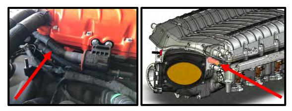
105. Install the supplied 3/8" ID x 24" brake aspirator hose from the brake booster to the **lower** quick connect fitting on the supercharger inlet. Push until it clicks into place. **TIP:** For best routing, nestle in between cam cover and fuel rail, under the wiring and heater hose.
