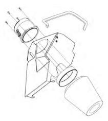
135. Install the factory MAF sensor element into the new MAF housing using the supplied (2) 4mm x 6mm SHCS. Torque to 17 lbs-in. **\*\*DO NOT USE STOCK BOLTS\*\*. \*TIP: Verify arrow position for airflow direction.**
