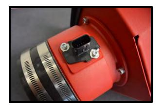
136. Install the high-flow air filter and clamp over the 123mm venturi ring. Once in place, secure hose clamp using a 5/16" nut driver. Drop airbox into position in vehicle. Secure box to frame by using the stock (2) plastic push pins at base of the box.
