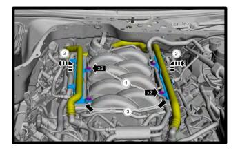
37. Loosen the 4 bolts holding the fuel rails down, these go through to the cylinder head (10mm socket). Fuel rail does not need to be removed.
