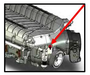
107. Install the supplied 5/8" ID x 9" hose to the passenger side valve cover. Connect other end to the supercharger inlet quick connect fitting. Push until it clicks and locks into place.
