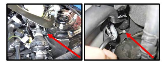
24. Disconnect and remove the positive crankcase ventilation PCV tube from inlet tube and LH cam cover fitting.
