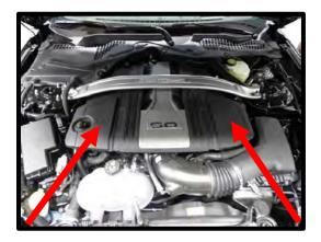
17. Remove the upper cowling for K-brace access. Remove the (7) push pin retainers and (2) tabs on the cowling. Lift up the cowl trim panel and remove the (4) nuts and (5) bolts from the K-Brace using a 13mm socket, remove from vehicle for later installation.
