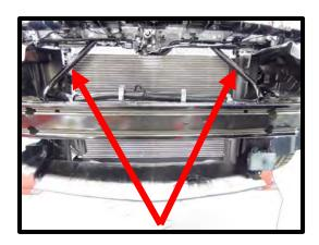
109. Using a panel puller, remove the (1) plastic pin holding the front snorkel to the radiator support. Using a hacksaw, cut the one side off as shown. Once cut, reinstall closeout using original plastic push pin.
