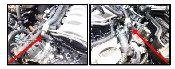
33. Disconnect the fuel psi sensor connector from driver side fuel rail.
