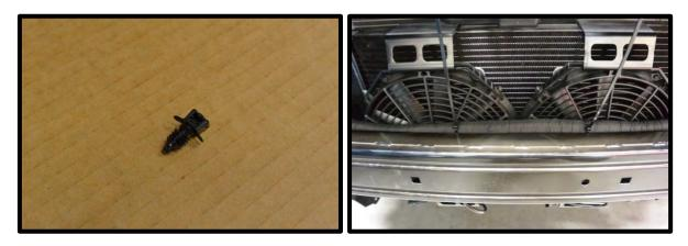
122. With the LTR mounted, mark the centerline of the LTR fitting and horizontally center of the plastic radiator (passenger side) shrouding. Using a 1 <sup>1</sup>/<sub>2</sub>" hole saw, drill a hole through the plastic shrouding. Install the supplied 1 <sup>1</sup>/<sub>2</sub>" rubber grommet into this hole. **NOTE:** Install hole and grommet as close to the plastic edge as possible. This gives proper clearance on the opposite side for the Y fitting.
