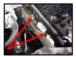
30. Carefully cut the electric tape securing the ETC wires to the throttle body. Disconnect the electronic throttle electrical connector by pushing up on the safety lock and then squeezing the connector and pulling away. Remove the harness support plastic tab from the block ground stud.
