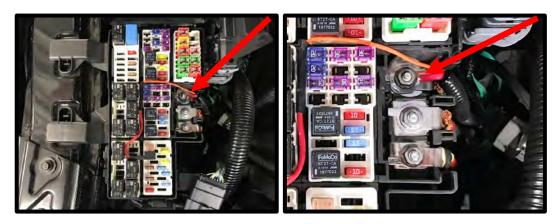
60. Pull the red 10amp fuse from position **#62** (ABS). Install the 10amp red fuse in the unused fuse slot on the fuse tap. Install the supplied fuse tap into position **#62** (ABS). **Note:** 10amp red fuse should be in bottom slot, 5amp should be in top slot. Make sure wire has enough room when fuse cover closes, route around fuses for clean installation.
