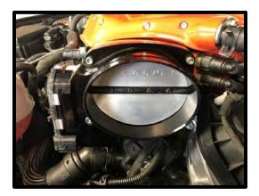
145. Install the supplied <sup>3</sup>/<sub>4</sub>" grommet into air inlet tube <sup>3</sup>/<sub>4</sub>" hole. Install the supplied <sup>1</sup>/<sub>2</sub>" to 5/8" quick connect aluminum fitting into grommet hole.
