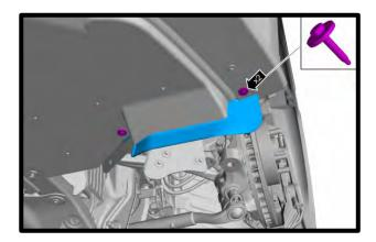
11. Remove the (19) lower close-out panel bolts (7mm socket) and the (2) push pins. Remove the lower close-out panel from vehicle.
