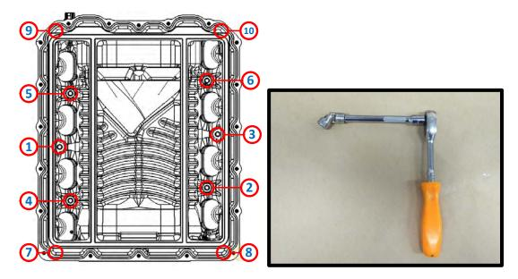
80. Install the supercharger pulley using the supplied (4) 6mm x 14mm SHCS using a 5mm allen socket. Leave hand tight until belt installation.
