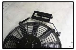
113. (**Dual fan installation**) Carefully set both fan assemblies on top front of the LTR, space these evenly before installing.
