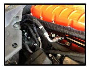
99. Connect the factory fuel inlet line to the driver side fuel fitting, press until it clicks and locks in place.
