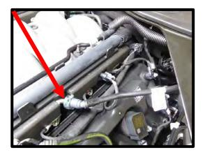
35. Using a 3/8" fuel line removal tool, remove the DI pump fuel feed line from PI fuel rail. *NOTE: THIS FUEL LINE HAS A CHECK VALVE, DO NOT FLIP ORIENTATION. DO NOT REMOVE FROM DI PUMP TO ELIMINATE CONFUSION. 90-DEG END ALWAYS CONNECTS TO FUEL FEED SUPPLY!*
