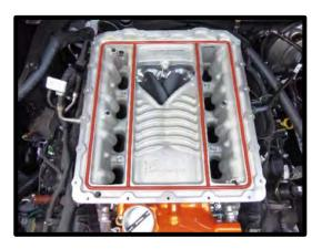
95. Install the supplied pre-formed 20.7" x .103" oring to the top sealing surface of the SC housing. Apply generous amount of grease to help ease the oring into place. **TIP:** To install oring into dove-tail groove, press vertically, vs sliding finger along.
