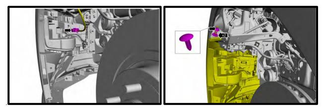
13. Carefully pull the fascia forward, disconnect the fog lamps before pulling away.
