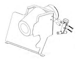
138. Connect the <sup>3</sup>/<sub>4</sub>" ID molded rubber hose you previously installed to the IC (**OUT**) fitting and connect to the IC filler neck. Secure with supplied pinch clamp.
