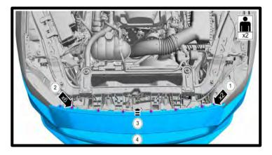
14. If equipped, disconnect the front active shutters electrical connector behind the bumper support. Remove the (6) plastic plush pins securing shutter assembly to front of vehicle as shown. These will not be reused. Wrap the connecter up, cover with electrical tape and secure with zip-tie to factory harness.
