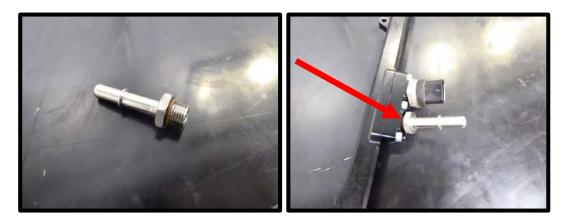
87. Install the supplied (1) #2-906 Viton oring to the (1 of 2) 45mm long 9.49mm outlet fitting. Apply light amount of grease to oring for ease of installation. Install fitting to the fuel inlet block. Install the supplied -6 ORB plug to the extra port.
