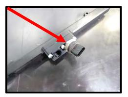
86. Install the supplied (1) #2-906 Viton oring to the (1 of 2) 45mm long 9.49mm inlet fitting. Apply light amount of grease to oring for ease of installation. Install fitting to the fuel inlet block.
