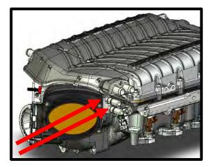
102. Mount the EECPV bracket to SC lid, use the (2) supplied 6mm x 10 HHFCS. Torque to 80 lbs-in using a 10mm socket.
