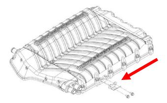
103. Slide the EECPV to bracket by sliding onto bracket. Connect factory plastic quick connect fitting to EECPV until it clicks and locks into place. Connect 2-way electrical connector to EECPV, press locking tab back in place.
