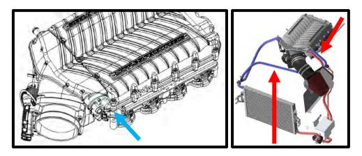
141. Install the (1) 5" ID x 2 <sup>1</sup>/<sub>2</sub>" silicone hose with dual #80 hose clamps to the MAF housing. Leave loose for now. \*\*Never over torque the clamp to secure the silicone hose to the MAF housing, this can distort the MAF and lead to running issues. 142. (Stock throttle body) Install throttle body adapter to supercharger inlet using the supplied (4) 6mm x 14mm FHCS (4mm allen socket) using the supplied gasket between TB adapter and SC inlet. Torque to 88 lbs-in.
