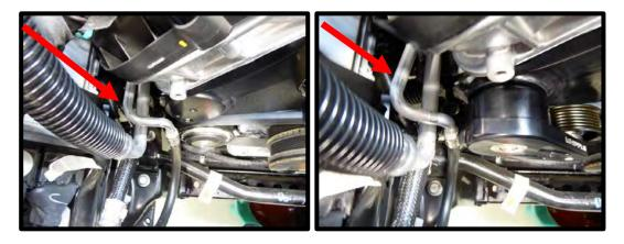
70. Install the spring-loaded tensioner to idler plate, locating the tang into position. Secure with the supplied (1) 10mm x 60mm SHCS. Use light amount of anti-seize on threads. Torque to 25 lbs-ft.
