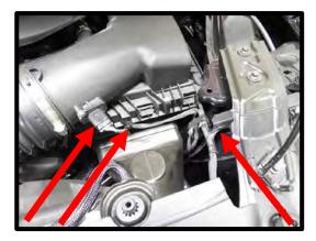
27. Loosen the factory air box lid by pushing the (2) locking tabs back. Loosen both hose clamps on the inlet tube (7mm nut driver). Remove tube, airbox lid and filter element from vehicle.
