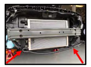
131. Install the supplied ¾" ID molded hose (#COYO-1300) from the IC OUT fitting to the airbox area for later installation. Secure end with supplied worm clamp. TIP: For hood clearance, ensure that the nut of the clamp is not on top.
