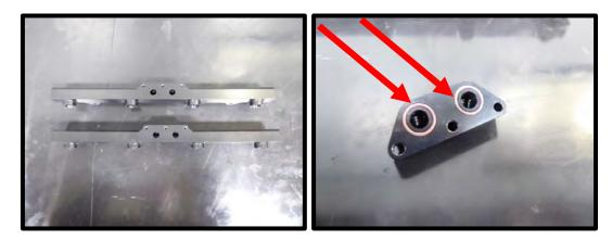
84. Using a 27mm socket, remove the fuel PSI sensor from the factory fuel rail. This will be reused at a later step.
