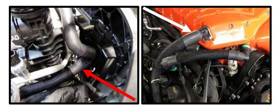
125. Install the supplied preformed <sup>3</sup>/<sub>4</sub>" x 48" dual 90deg hose #3102698 to upper Y fitting and secure with pinch clamp. Route up and over the condenser to LH side of vehicle. Leave this end loose until airbox installation. Secure hose to factory holes using zip-tie to prevent hose from sitting on AC Condenser.
