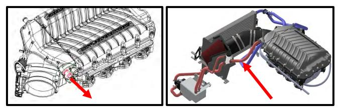
139. Install the supplied 3/8" ID x 31 ½" IC vent line (COYO-1400) and the 3/4" ID x 24 ½" IC rubber hose (COYO-1300) to the filler neck. Both use the 90deg on the filler tee. Secure both with supplied pinch clamps. Route both below the airbox, to the IC reservoir. Secure both ends with supplied pinch clamps. Use multiple zip-ties to secure hoses together. Watch for hose kinks!
