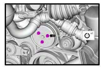
44. Remove the belt from the engine by using a 15mm socket on a  $\frac{1}{2}$ " breaker bar and rotating the spring-loaded tensioner in a clockwise direction.
