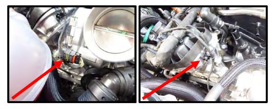
31. Remove the vent hose coming from the thermostat housing fitting by removing pinch clamp. Remove vent line from overflow tank by removing pinch clamp using a pinch clamp tool. This hose will not be reused.
