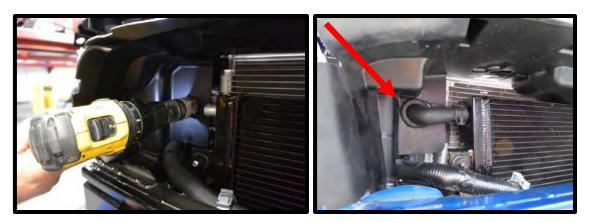
123. Route the supplied 90deg intercooler feed hose #COYO-2006 through the grommet, cut to fit as needed. Install the supplied Y fitting to the end of the hose from the outlet of the LTR, just after the grommet. Secure hose to fitting with pinch clamp.
