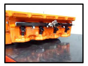
91. Install the supplied fuel cross over line around the back of the supercharger by pressing until they click and lock in place.
