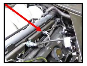
34. Carefully disconnect the factory fuel feed hose from the fuel rail. The fuel system may still have pressure, use protective eyewear and multiple rags to catch any possible fuel leak. To release, press the blue safety latch and pull the fuel fitting away from fuel rail.
