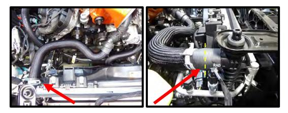
56. Remove the coolant vent hose from the radiator and pull back the plastic sheaving. Shorten this hose end by 1" for additional clearance. Reinstall hose using factory clamp.
