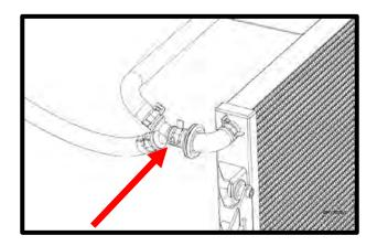
124. Connect the <sup>3</sup>/<sub>4</sub>" x 34.5" #3102697 hose to the Y fitting, secure with pinch clamp. Route other end to the RH side of the water cross fitting. Secure with the supplied worm clamp. For max hood clearance, ensure that the hex is not on top.
