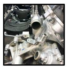
50. Install the supplied tee and 90deg hose to the driver side heater tube you just installed. Secure with the supplied pinch clamp on the 90deg hose to heater tube. **NOTE:** Short end of 90deg goes on heater tube, long end goes on tee fitting.
