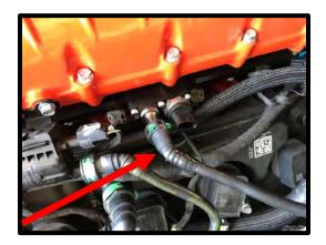
100. Connect the factory fuel PSI sensor connector to sensor, press safety lock until it clicks and locks in place.
