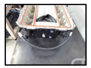
92. Install the supplied ¼" ID bypass actuator to the bypass nipple and ¼" nipple on SC housing. **CAUTION:** Do not open/close bypass actuator by hand. This may damage actuator internally. It only moves properly with equal vacuum/boost at the actuator reference port. **NOTE: Install zip tie to 90deg rubber fitting on bypass actuator nipple to secure.**
