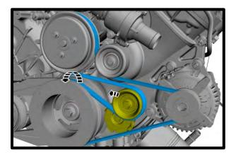
45. Remove the spring-loaded tensioner from the engine using a 13mm socket.
