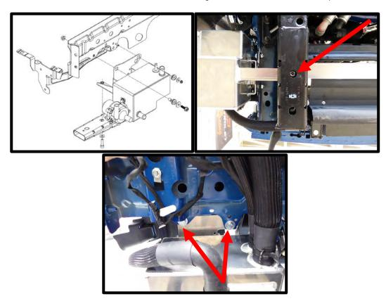
128. (Standard LTR) Using a hacksaw, notch the plastic shrouding next the heat exchanger inlet fitting. Use the supplied 3/4" ID x 20" hose with 90deg end for test fitting (from pump outlet to LTR inlet).
