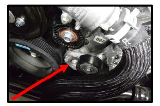
46. Remove the water pump pulley using a 10mm socket (this will be reused).
