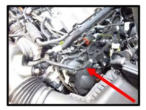
25. Disconnect the green connector from the evaporative emission canister purge valve (EECPV) tube and the electrical connector. Disconnect green connector securing EECPV line to intake manifold. Lift EECPV purge valve from intake manifold for later use. Remove the plastic line from the EECPV purge valve by carefully cutting plastic line. **NOTE:** Do not cut oring under plastic hose.
