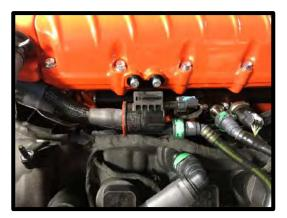
104. Install the supplied 3/8" ID x 5 ½" hose to the EECPV barb fitting and **upper** quick connect fitting on SC inlet. Push until it clicks and locks into place.
