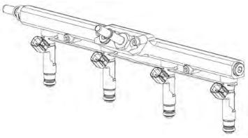
90. Apply generous amount of grease to the injector orings for ease of installation. Install the fuel injectors, rails and lock bracket to the intake manifold, secure with the (4) 6mm x 20mm SHCS using a 5mm allen socket. Torque to 90 lbs-in.
