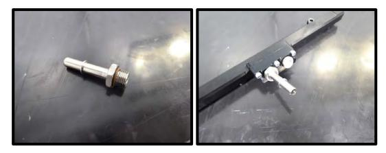
88. Install the supplied (2) #2-906 orings to the (2) inlet/outlet fittings. Install these (2) fittings into rear side of fuel rails. Apply light amount of grease to oring for ease of installation. Using a <sup>3</sup>/<sub>4</sub>" wrench (or <sup>3</sup>/<sub>4</sub>" deep socket) on both the front and rear fittings, tighten both.
