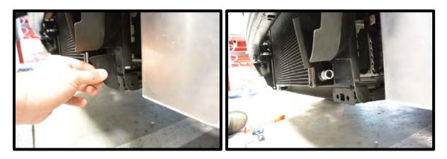
129. (Standard LTR) Route the <sup>3</sup>/<sub>4</sub>" ID x 16" hose from IC pump outlet to LTR inlet. This hose has to go up and towards the tank as shown in the image. Failure to do so may cause clearance issues.
