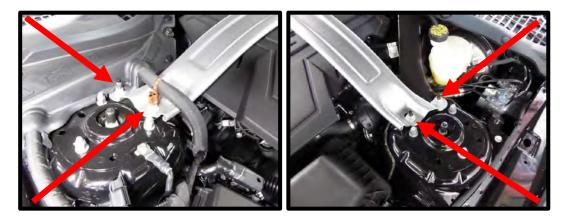
16. Using a flat head screw driver, remove the (2) plastic cups exposing the fasteners below. Using a 10mm socket, remove the (2) bolts securing cover to engine. Lift and remove cover from the engine.
