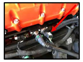
101. Install the (2) supplied 6AN viton oring (#906) to the (2) 6AN to 3/8" quick connect fittings. Install these fittings to the passenger side lower 6AN fittings on the inlet using an 11/16" socket.
