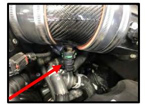
147. Connect the previously routed ¼" vent line to the stock overflow tank, secure with stock clamp. Secure this hose to the radiator hose and heater hose using multiple zip-ties.
