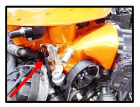
93. (Complete Kits Only) Connect the previously installed ACT pigtail (IAT2 manifold air temperature) to the preinstalled ACT sensor located on the driver side of intake manifold. Competition Kits: ACT pigtails are not included. Contact your tuning shop for proper wiring and sensor if you want to add post intercooler temps to PCM.
