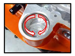
97. Apply generous amount of grease to the (1) #2-230 Viton bypass oring. Install the supercharger lid to the supercharger housing by carefully placing the bypass down. Secure the SC lid using the (17) 6mm x 30mm HHFCS and (3) 6mm x 70mm HHFCS (*marked green*) using the following pattern. Torque to 90 lbs-in using an 8mm socket.
