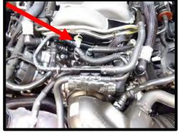
22. Using a pinch clamp tool, remove the brake booster line that connects the brake aspirator rubber line to hard line.
