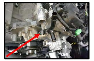
43. Loosen the (3) bolts securing the water pump pulley (while belt is on) using a 10mm socket.
