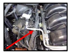
36. Remove the (4) nuts from the top of the intake manifold that secures the (2) heater hose trays and brake aspirator line. Use a 10mm deep well socket. Once bolts are removed, remove tray, brake aspirator and foam material.
