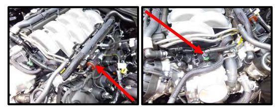
26. Disconnect the MAF connector by pulling back on the safety lock, then squeezing the unlocking tab and pulling back. Using a panel puller tool, remove the wiring harness support tab from the airbox.
