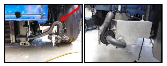
130. (HD LTR) Use the supplied <sup>3</sup>/<sub>4</sub>" coupler and (2) pinch clamps to couple the <sup>3</sup>/<sub>4</sub>" x 20" hose to the <sup>3</sup>/<sub>4</sub>" x 31" extension. Route the 180deg end to the LTR inlet. Secure using pinch clamp.
