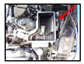
29. Pull the (2) push pins securing the engine harness to the frame on the driver side, this will be reused later to secure the airbox.
