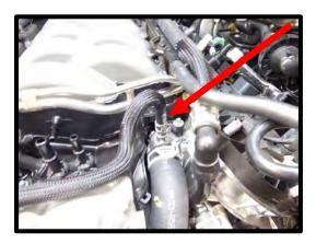
32. Remove the heater hose from both driver and passenger side of block by pulling locking tab back and pulling away. Push to the back of the engine for later use.
