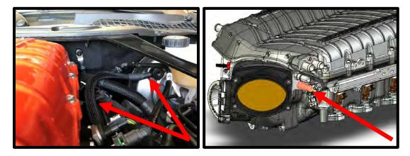
106. Install the (1) supplied 6AN viton oring (#906) to the (1) 6AN to 5/8" quick connect fittings. Install this fitting to the driver side 6AN fittings on the inlet using a 7/8" wrench.
