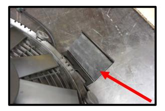
112. (**Dual fan installation**) Install the (4) brackets to the fans by sliding the square tab into the fan notch and the steel channel bracket will slide on the outside. The angled side will face the fan. This slides together easier if the bracket is facing slightly up. Once these are lined up, push until the seat together. Repeat on the other (3) brackets. Leave nyloc nuts loose for now.
