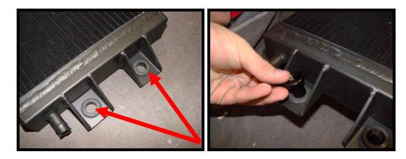
117. Install the LTR brackets to the LTR using the supplied (4) 8mm x 35mm FHSCS bolts through the aluminum heat exchanger spuds (5mm allen socket).
