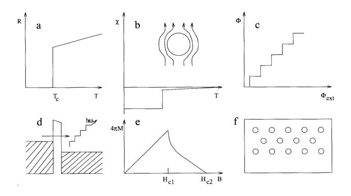
Fig.2. Basic properties of superconductors. (a) Zero resistance, (b) Meissner effect, (c) flux quantization, (d)Josephson effect, (e,f) mixed state and Abrikosov vortices.
