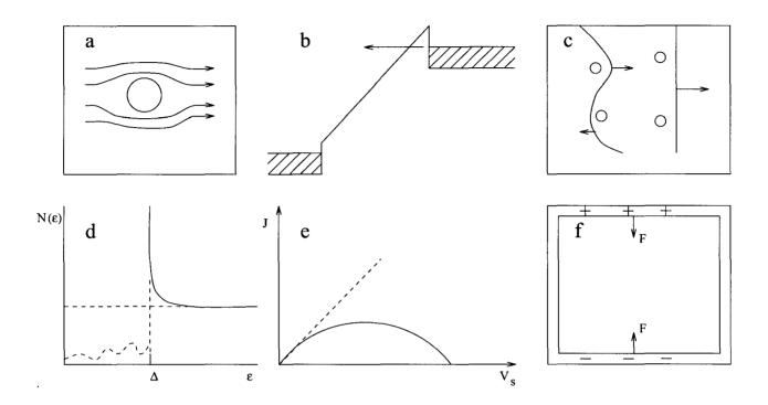
Fig.5. Phenomena near the superconducting surface related to RF losses. (a)Supercurents bypassing a non-superconducting inclusion, (b) cold electron emission from the metal, (c) oscillation and depinning of trapped vortices, (d) quasiparticle states inside superconducting energy gap, (e) depairing mechanism, (f) deformation of the cavity wall.
