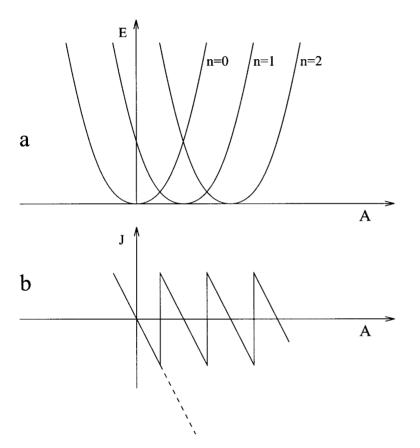
**Fig.4.** Energy vs vector potential (a) and current vs vector potential (b) dependences in a hollow superconducting cylinder. Solid line in (b) corresponds to the persistent current in the cylinder wall, dashed line to a supercurrent.
