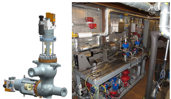
Figure 6 – Turbine Stop Valve and Stem Testing at GE-GR
