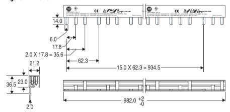
Figure 22 - Auxiliary Contacts — 1492-ASPHH3, ASPHS3, ASPH3, AS9HSC3P
