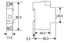
Figure 24 - Shunt Trip Module — 1492-ASPA
