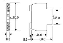
Figure 23 - Undervoltage Release Module — 1492-ASPU
