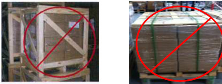
Figure 21 - Incorrect Usage of Wooden Materials [1].
