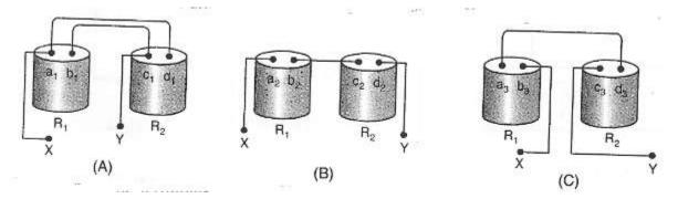
They connect the terminals marked X and Y above to the terminals marked X and Y in the given circuit. They record the ammeter readings (I) for different positions of the rheostat and the corresponding voltmeter readings (V).
