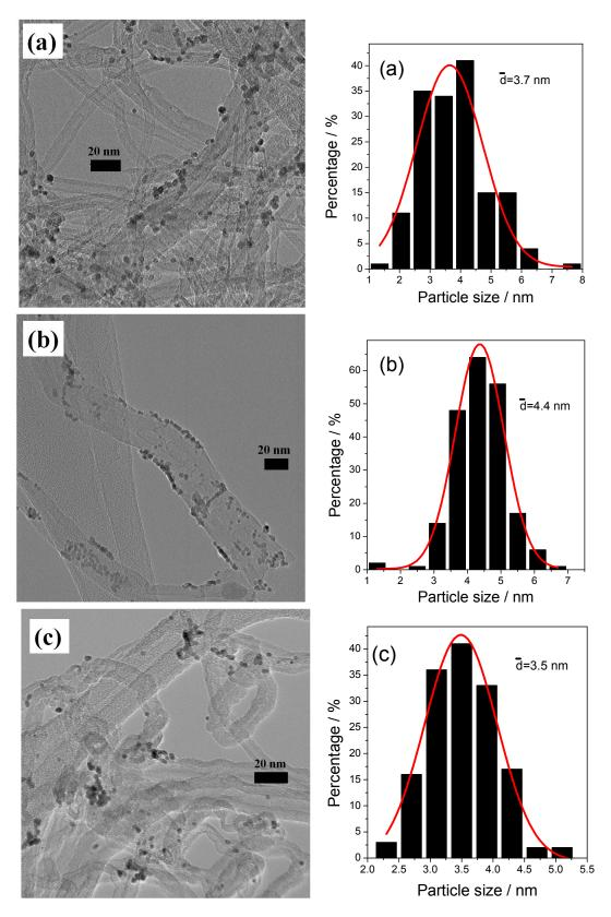
Fig. S7 TEM micrographs and size distributions: (a) Fe/CNT; (b) PtFe/CNT; (c)  $FeO_x/Pt/CNT$
