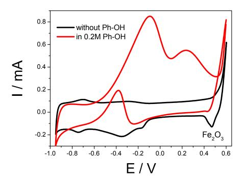
Fig. S3 Cyclic voltammograms (50mV/s) for FeO $_x$ /Pt/CNT in 0.1M KOH and in 0.1M KOH + 0.2 M benzyl alcohol
