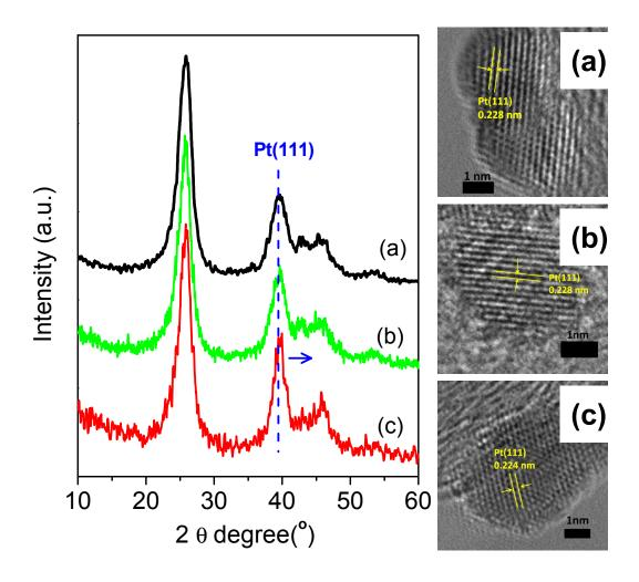
**Fig. S1** XRD patterns (left) and HRTEM images (right) of Pt/CNT (a), FeO<sub>x</sub>/Pt/CNT (b) and PtFe/CNT (c)
