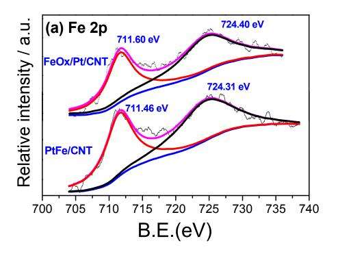
Fig. S4 Fe 2p XPS spectra of FeO<sub>x</sub>/Pt/CNT and PtFe/CNT
