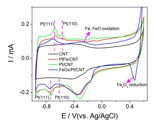
Fig. S2 Cyclic voltammograms (50 mV/s) for different samples in N<sub>2</sub> purged 0.1 M KOH, under room temperature
