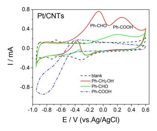
Fig. S5 Cyclic voltammograms (50 mV/s) for Pt/CNT in 0.1M KOH and 0.2 M different reactants, under room temperature, with  $N_2$  saturated
