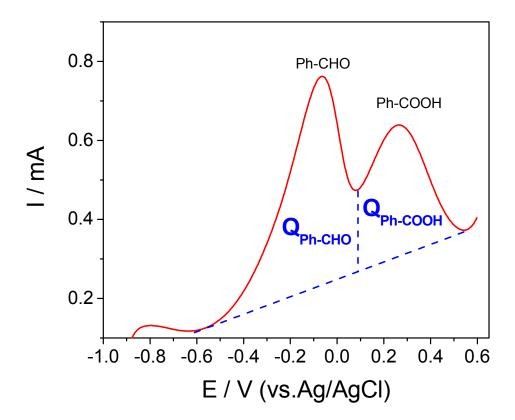
Fig. S6 Potentiodynamic current of benzyl alcohol electro-oxidation on Pt/CNT in 0.1M KOH and 0.2 M benzyl alcohol, under room temperature, with  $N_2$  saturated, scan rate = 50 mV/s
